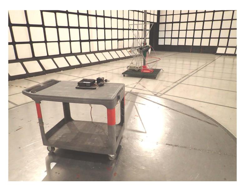
Transmitter Radiated Emission Test at 3m, above 1GHz
