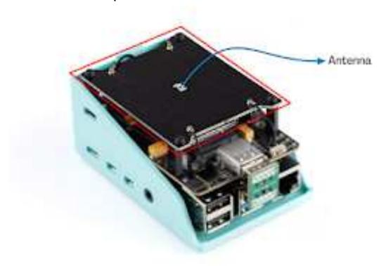
This antenna has been specifically designed and produced by Sixfab engineers, focusing on 5G bands and frequencies, exclusively for the Jumpstart 5G product.
