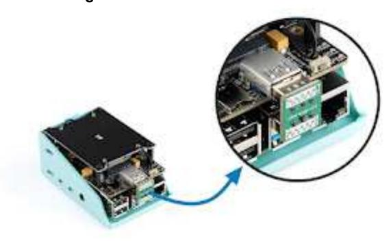
The USB Bridge serves the purpose of connecting the 5G module with the USB 3.0 port of the Raspberry Pi. This design choice was made in favor of using a USB cable, as it provides a robust, aesthetic, and space-saving solution. Rather than a standard straight cable connection, the USB Bridge has been specifically designed with EMI/EMC filtering components to ensure faster and more efficient data transmission.
