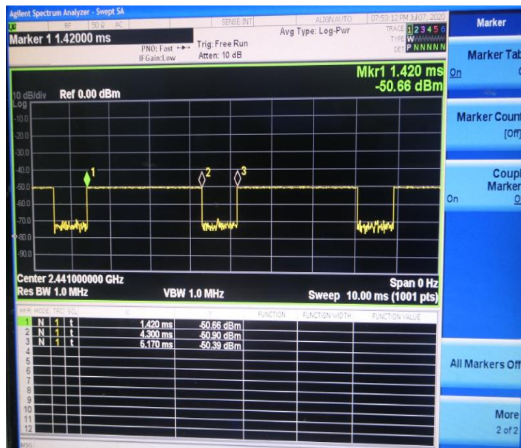
Time-domain plot for Bluetooth transmission signal
