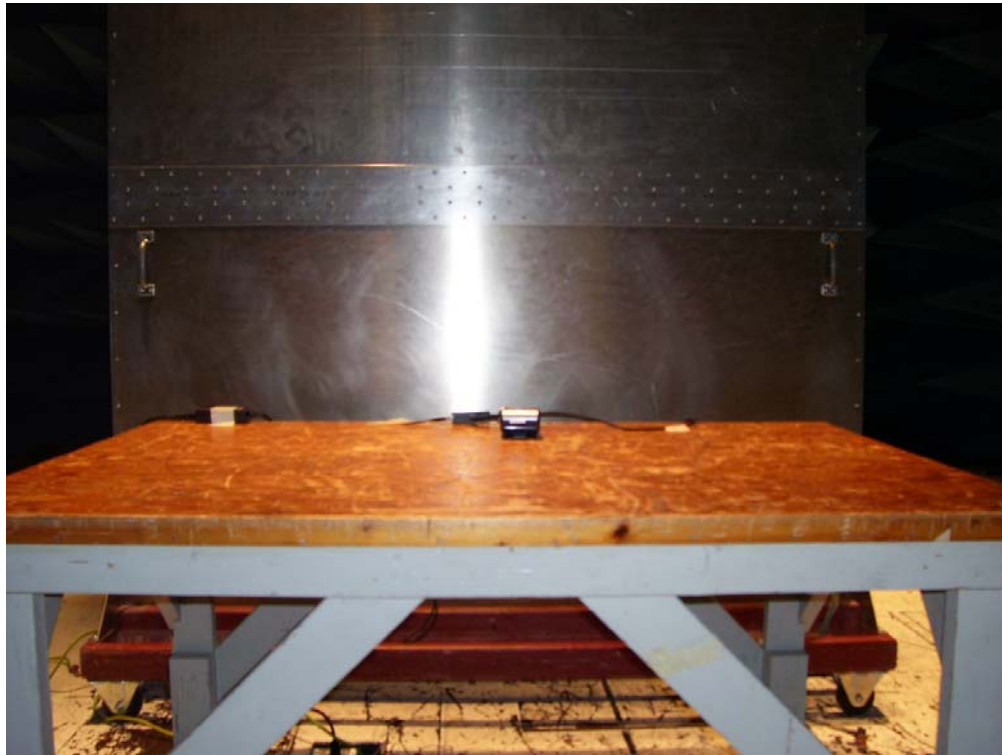
Photograph 2. Conducted Emissions Test Setup
