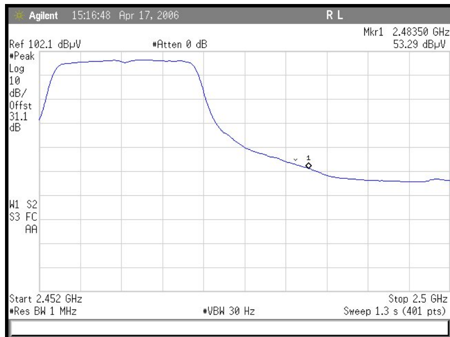
Plot 14. OFDM Radiated Restricted Band 2483.5 MHz – 2500 MHz Average
