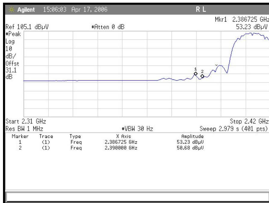
Plot 8. DSSS Radiated Restricted Band 2310 MHz – 2390 MHz Average
