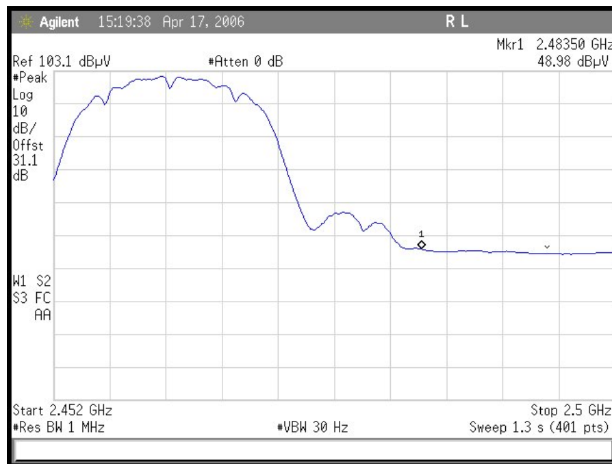
Plot 10. DSSS Radiated Restricted Band 2483.5 MHz – 2500 MHz Average
