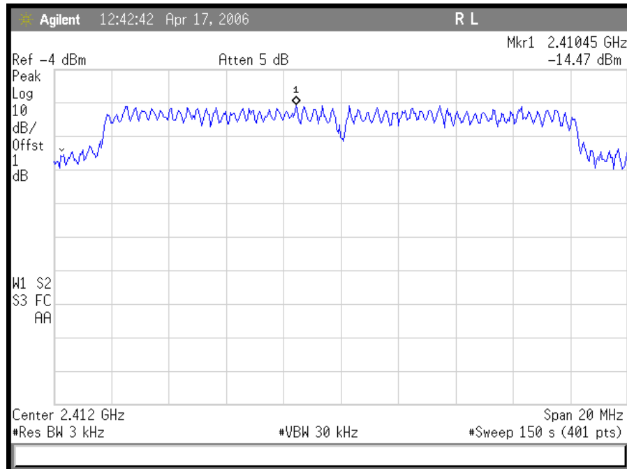
Plot 34. 802.11/g – OFDM Low Ch Peak Power Spectral Density
