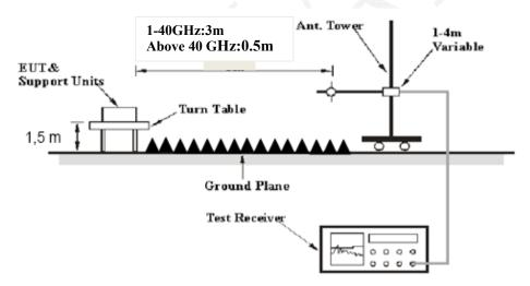
The radiated emission and out of band emission tests were performed in the 3 meters chamber test site, using the setup accordance with the ANSI C63.10-2013 The specification used was the FCC 15.209/15.205 and FCC 15.255 limits.
