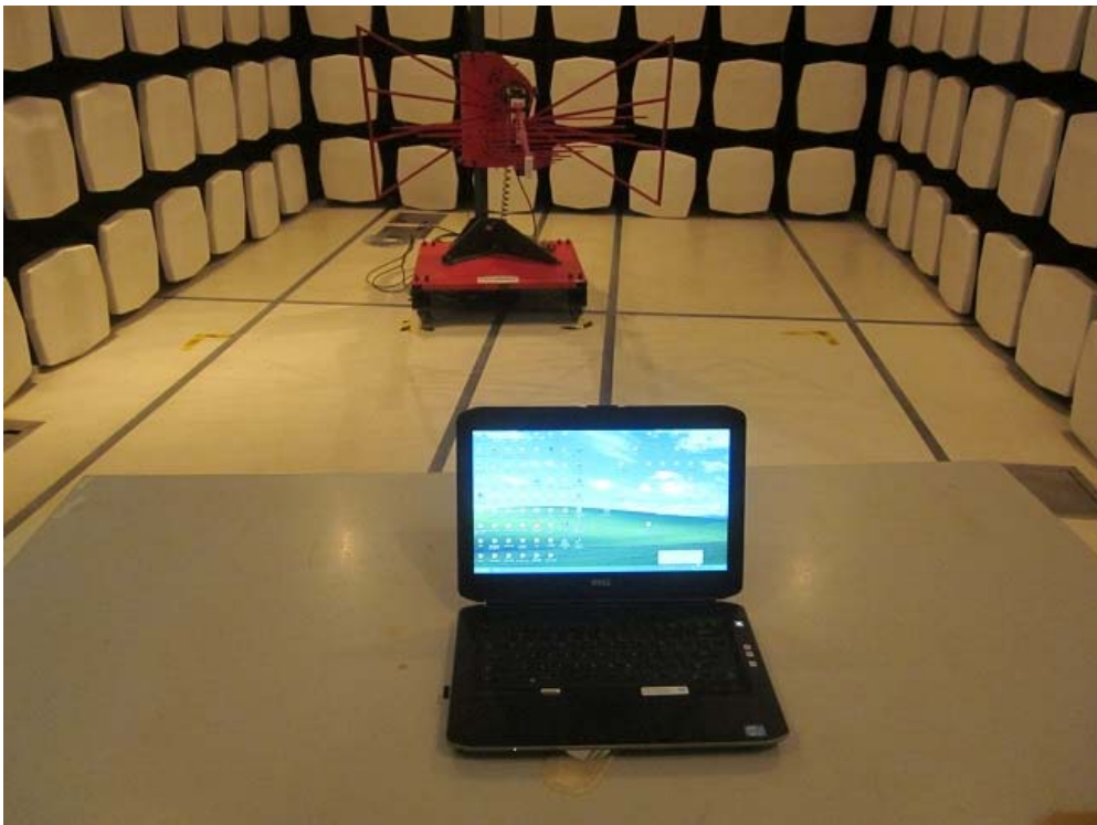
Measurement of Radiated Emission Test Set Up
