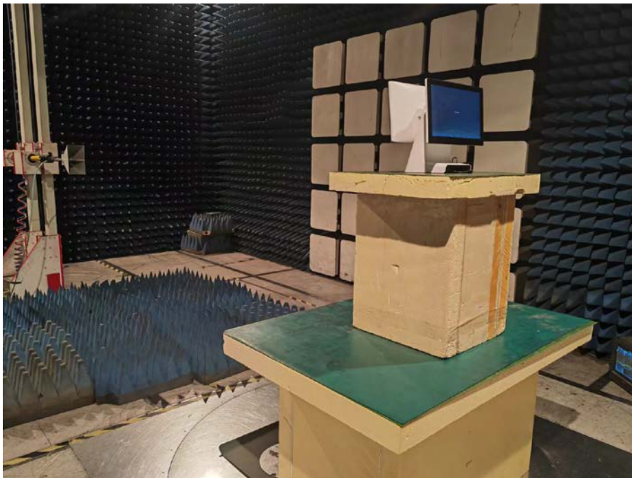
Spurious Emission Test Setup (Above 1GHz)
