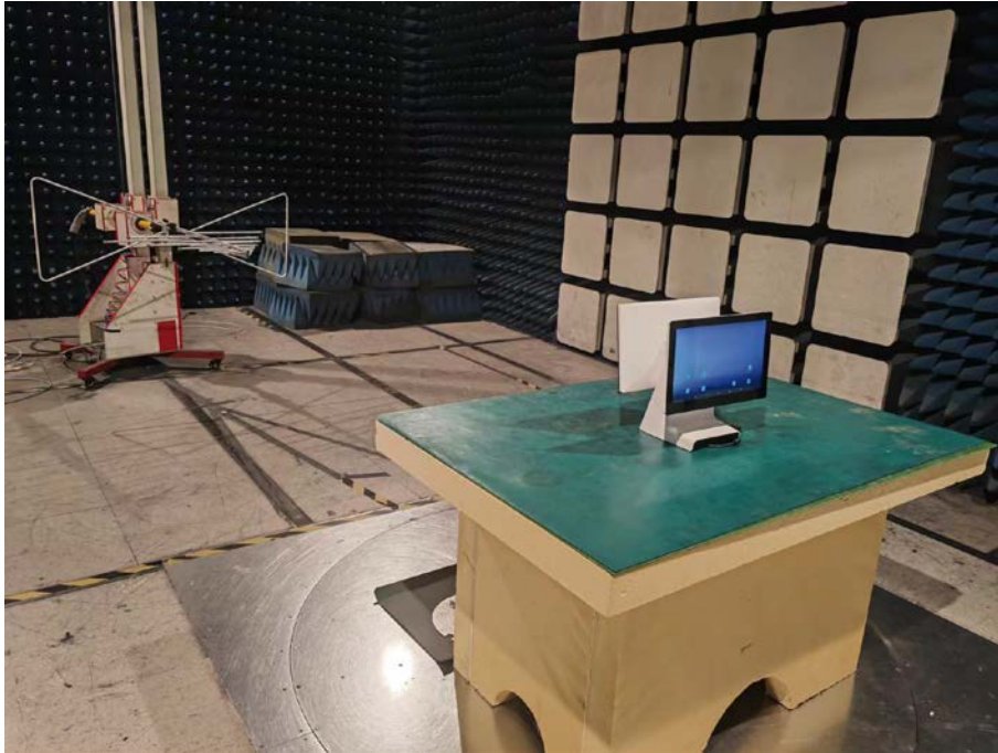
Spurious Emission Test Setup (Below 1GHz)
