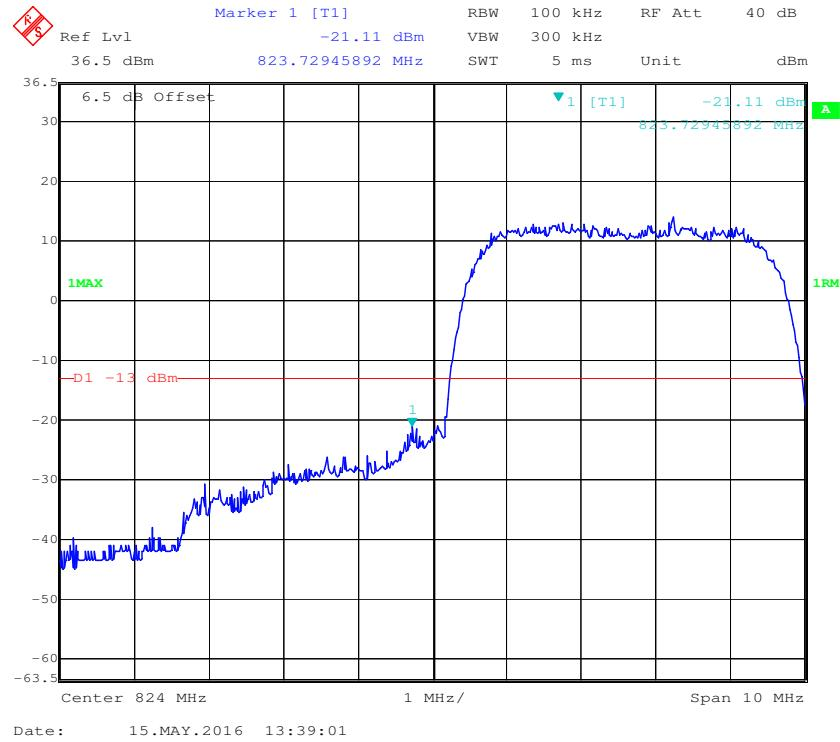
**Cellular Band, Right Band Edge for HSUPA (BPSK) Mode**
