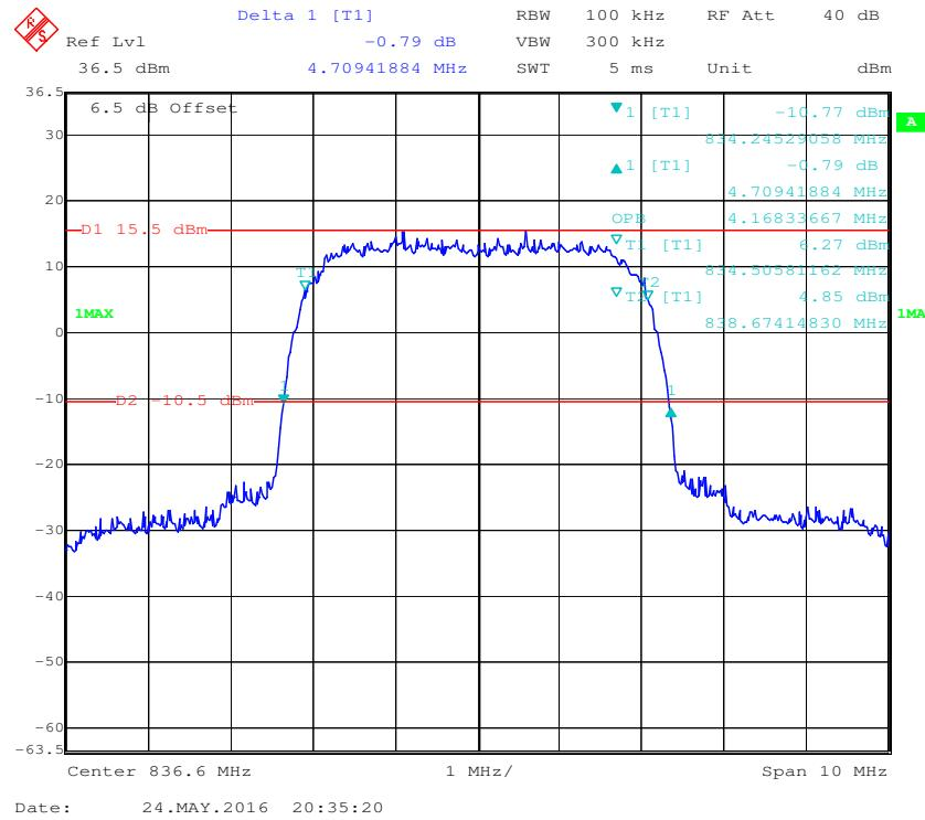
**99% Occupied & 26 dB Emissions Bandwidth for HSDPA (16QAM) Mode**
