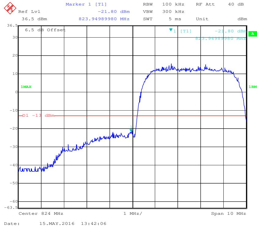
**Cellular Band, Right Band Edge for WCDMA (BPSK) Mode**
