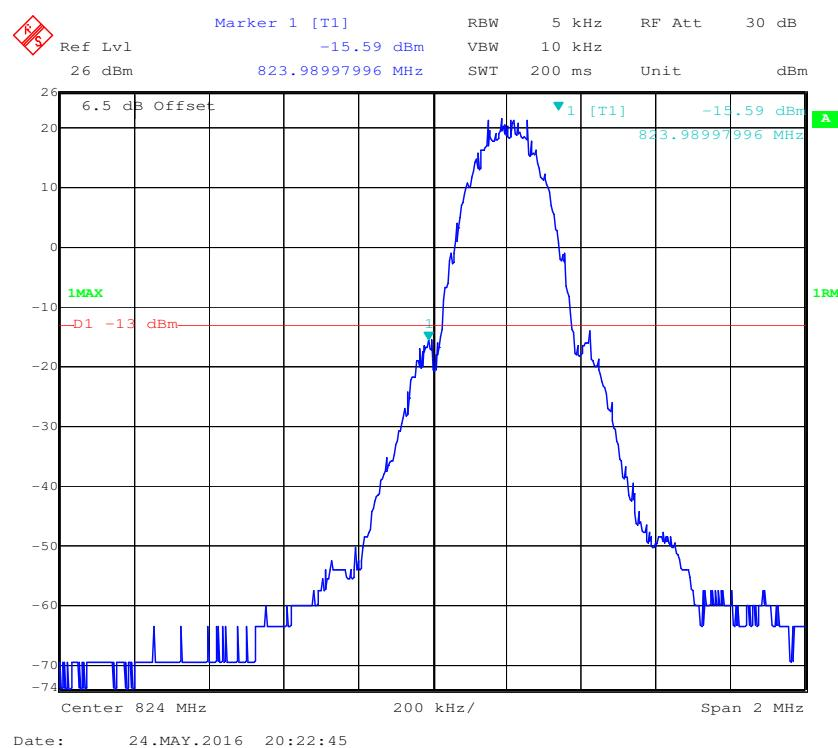
**Cellular Band, Right Band Edge for GSM (GMSK) Mode**
