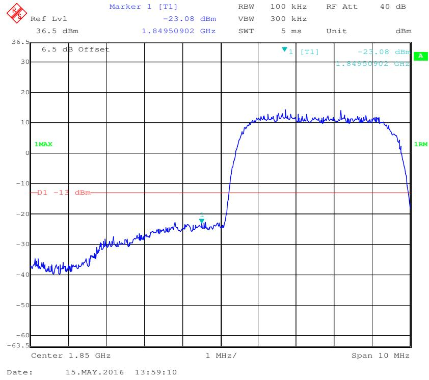
**PCS Band, Right Band Edge for WCDMA (BPSK) Mode**
