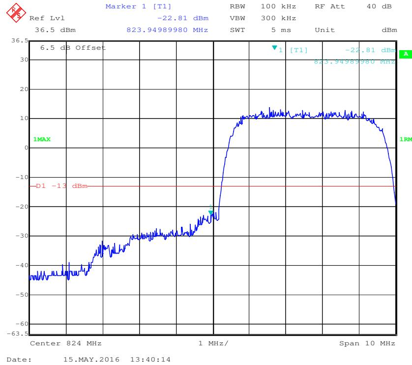
**Cellular Band, Right Band Edge for HSDPA (16QAM) Mode**
