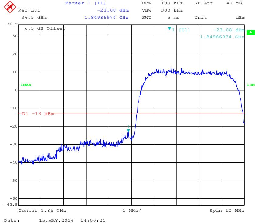
**PCS Band, Right Band Edge for HSDPA (16QAM) Mode**
