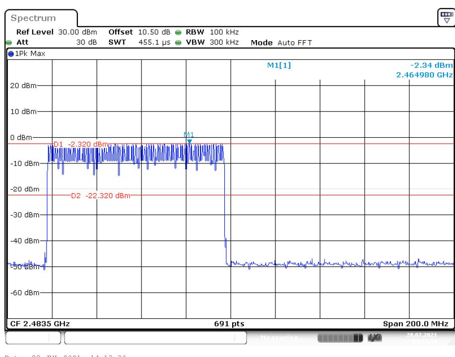
**EDR (8DPSK): Band Edge-Left Side****Single**
