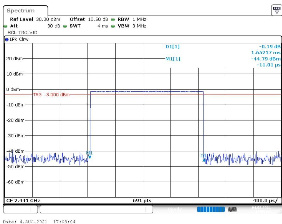
**Pulse time, DH5**
