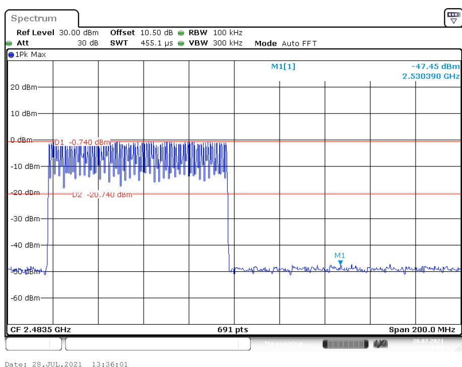
**EDR ( $\pi/4$ -DQPSK): Band Edge-Left Side****Single**
