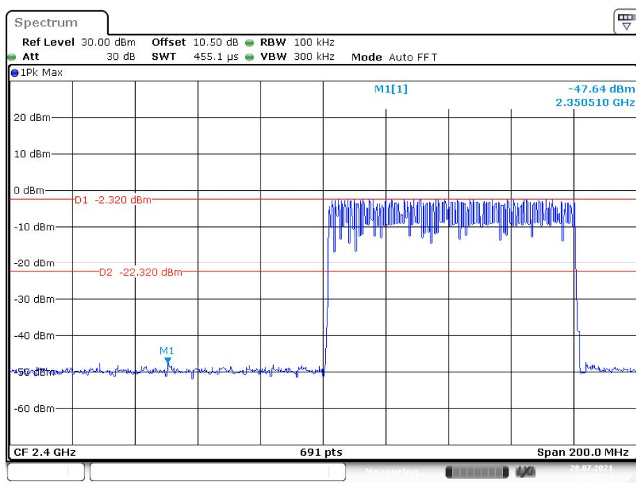
**EDR ( $\pi/4$ -DQPSK): Band Edge-Right Side****Single**
