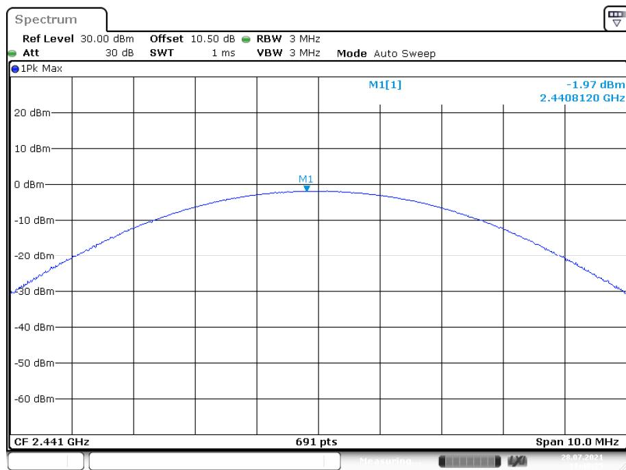
**EDR ( $\pi/4$ -DQPSK): High Channel**
