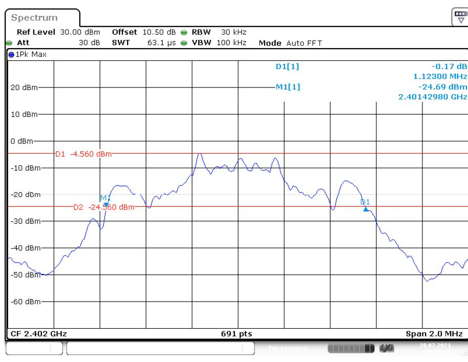
**EDR ( $\pi/4$ -DQPSK): Middle Channel**
