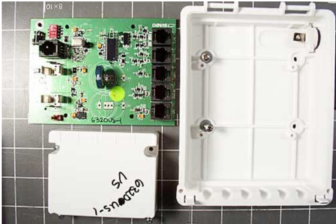
RF PCB Removed from Plastic Enclosure
