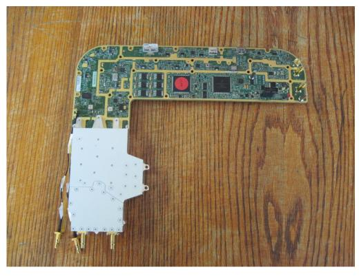
RF cavity filter with cover removed that is connected to end of PCB
