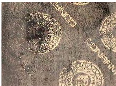
Figure 5: Damaged 3M™ Confirm™ Laminate
