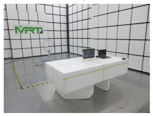
Description: Radiated Emission Test Setup for above 30MHz
