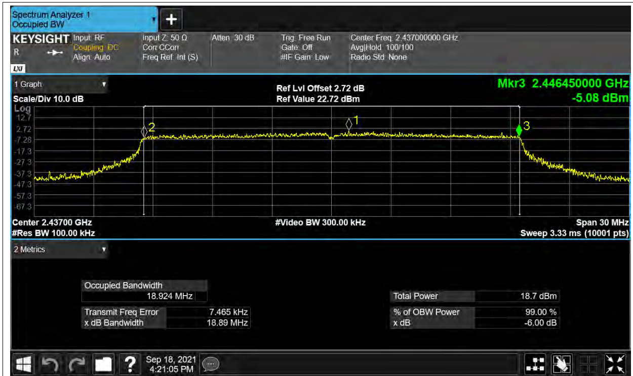
-6dB Bandwidth NVNT ax20 2437MHz ANT2
