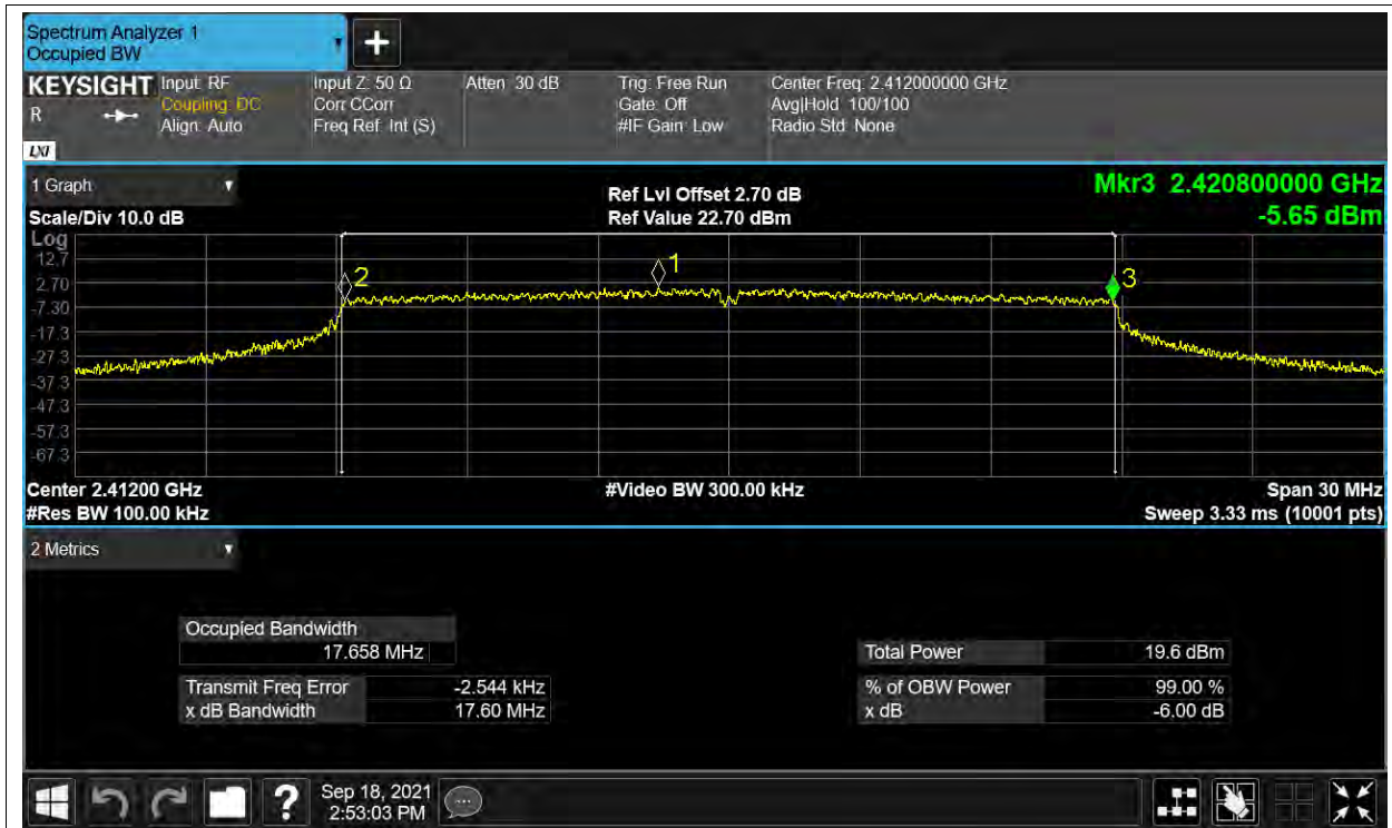
-6dB Bandwidth NVNT n20 2412MHz ANT2
