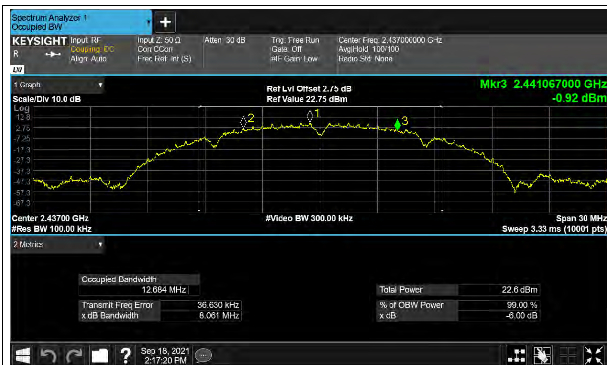
-6dB Bandwidth NVNT b 2462MHz ANT2
