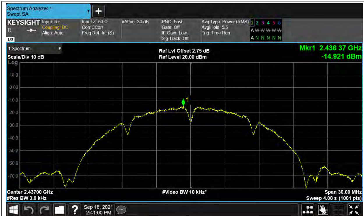
PSD NVNT b 2462MHz ANT2
