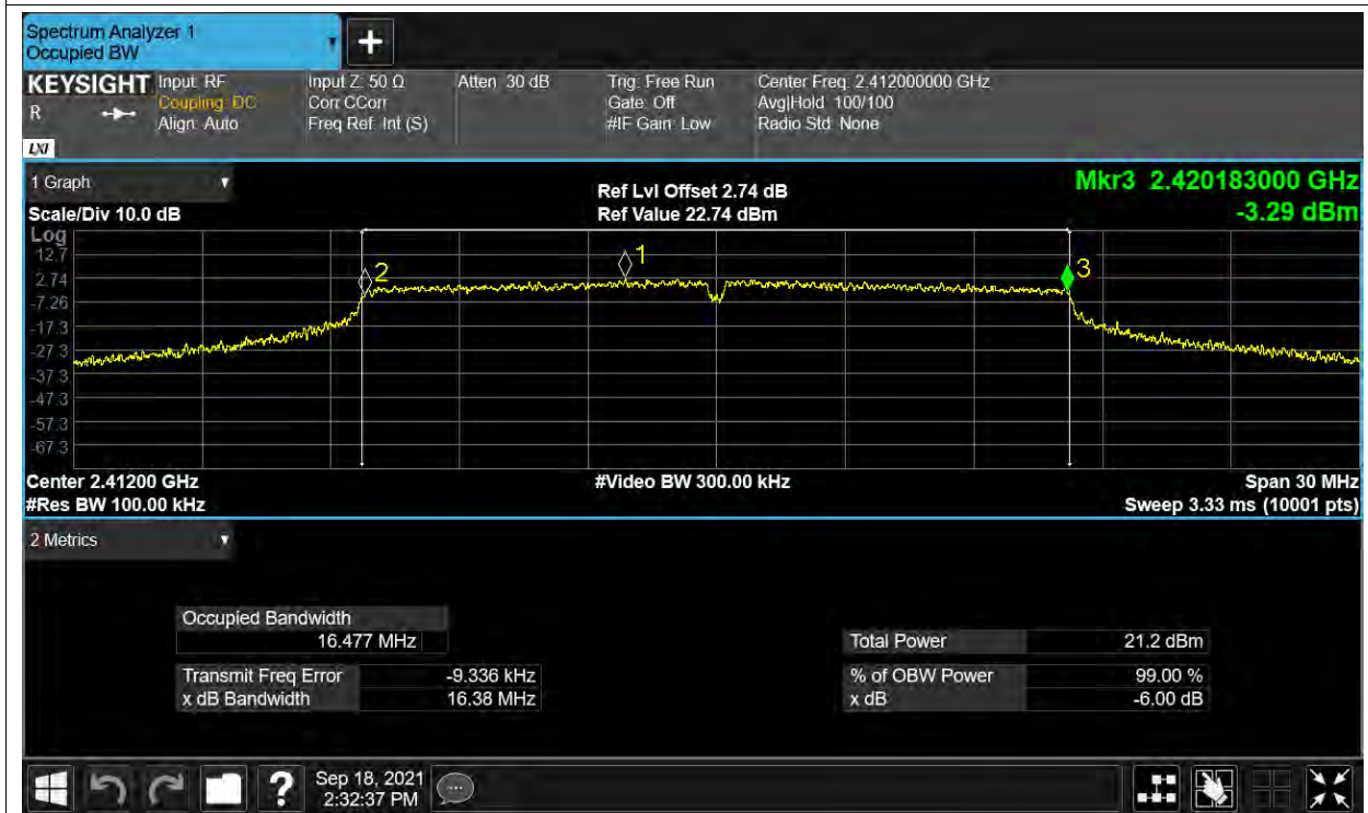
-6dB Bandwidth NVNT g 2437MHz ANT2
