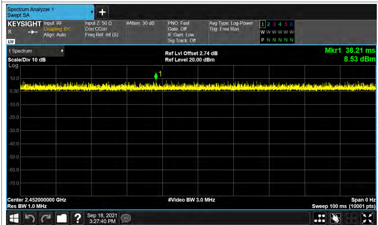
Duty Cycle NVNT n40 2452MHz MIMO
