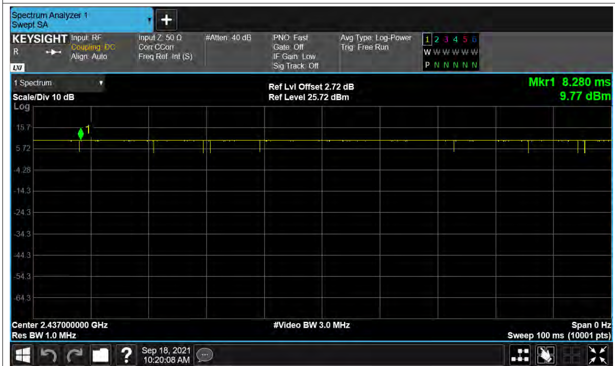
Duty Cycle NVNT b 2462MHz ANT1
