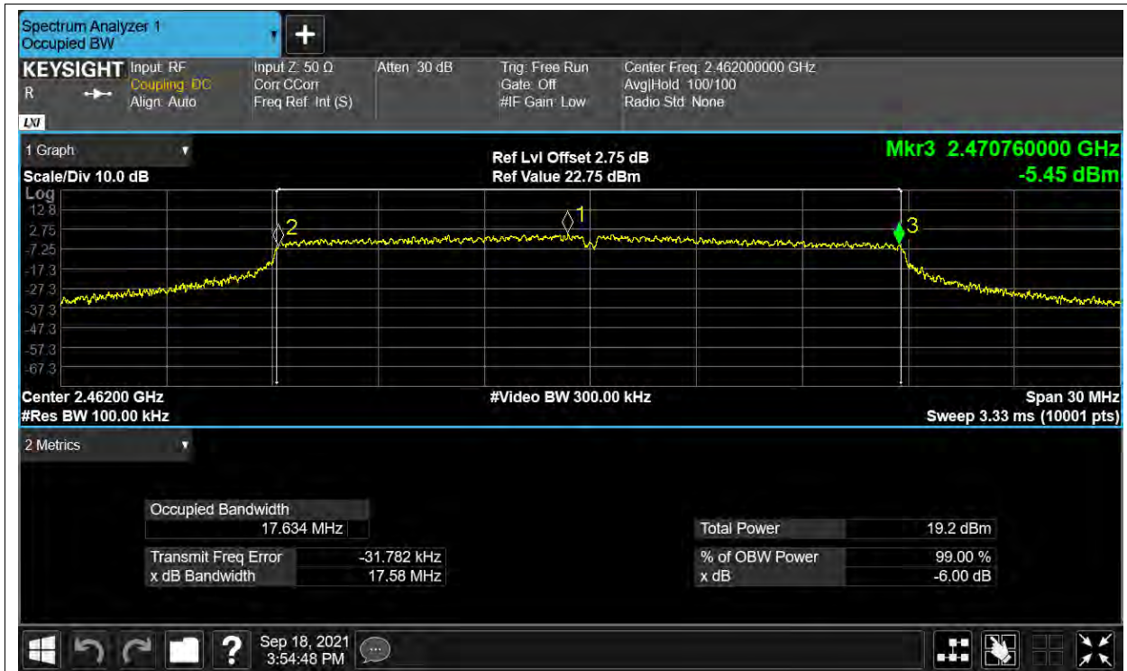
-6dB Bandwidth NVNT n20 2462MHz ANT2
