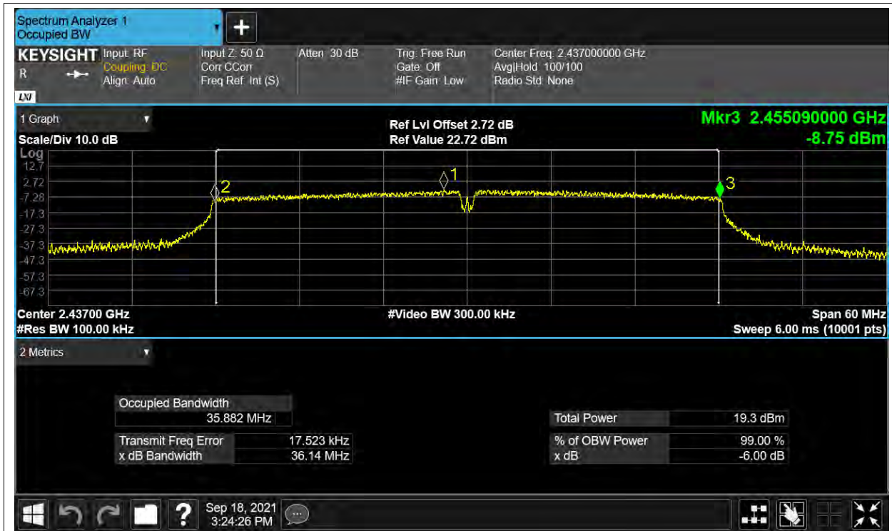
-6dB Bandwidth NVNT n40 2437MHz ANT2
