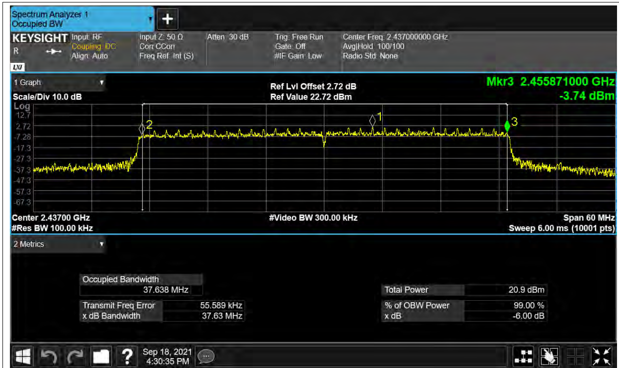
-6dB Bandwidth NVNT ax40 2437MHz ANT2
