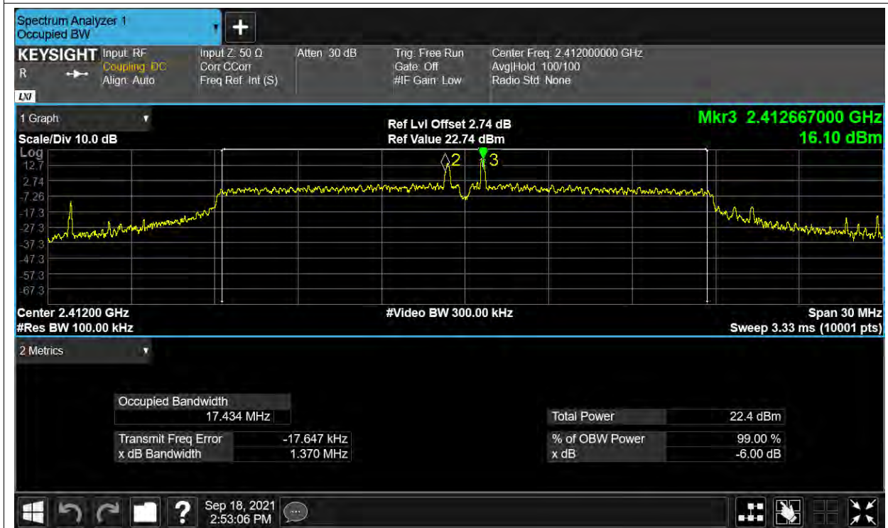
-6dB Bandwidth NVNT n20 2437MHz ANT1
