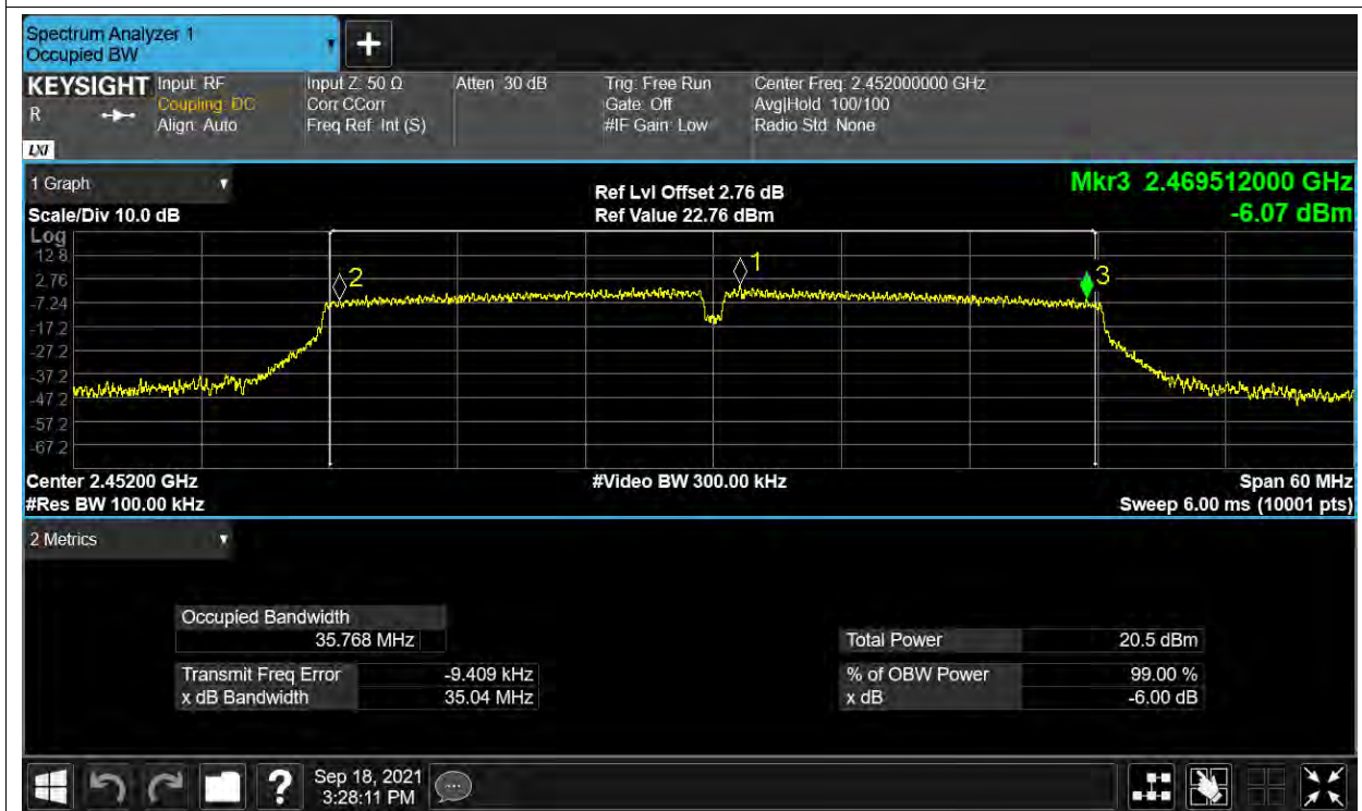
-6dB Bandwidth NVNT n40 2452MHz ANT2
