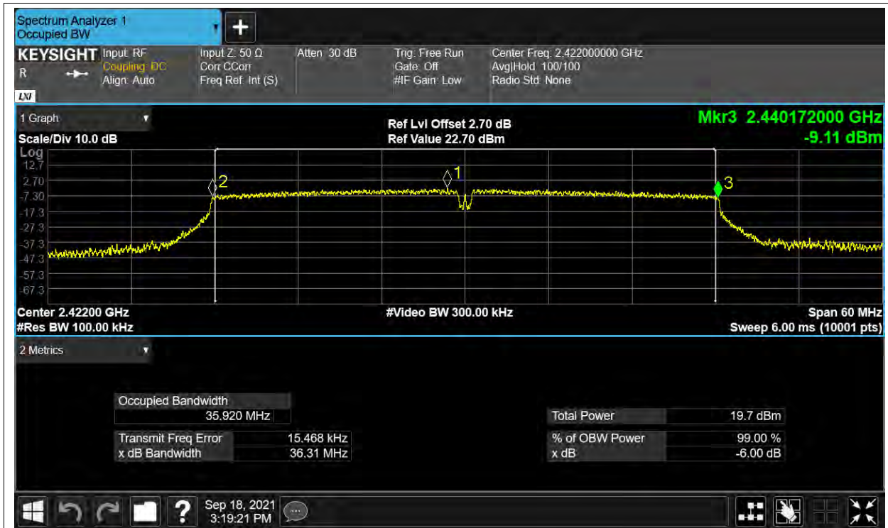
-6dB Bandwidth NVNT n40 2422MHz ANT2
