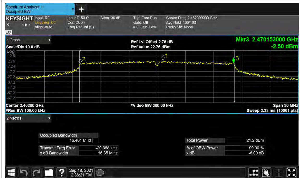
-6dB Bandwidth NVNT n20 2412MHz ANT1
