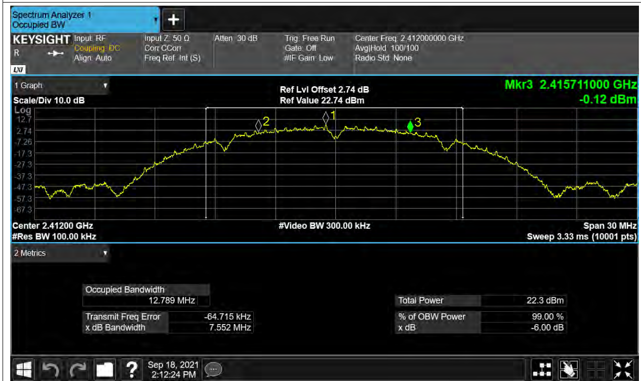
-6dB Bandwidth NVNT b 2437MHz ANT2
