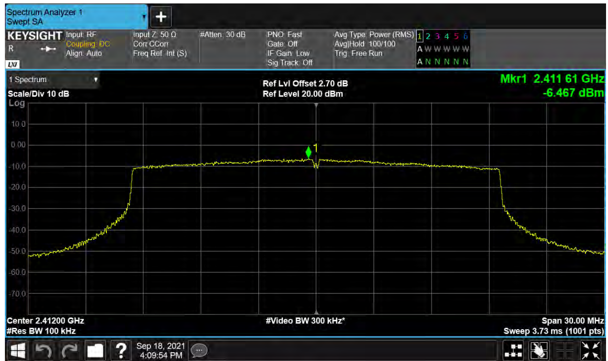
PSD NVNT ax20 2412MHz ANT2
