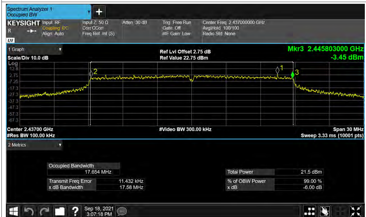
-6dB Bandwidth NVNT n20 2462MHz ANT1
