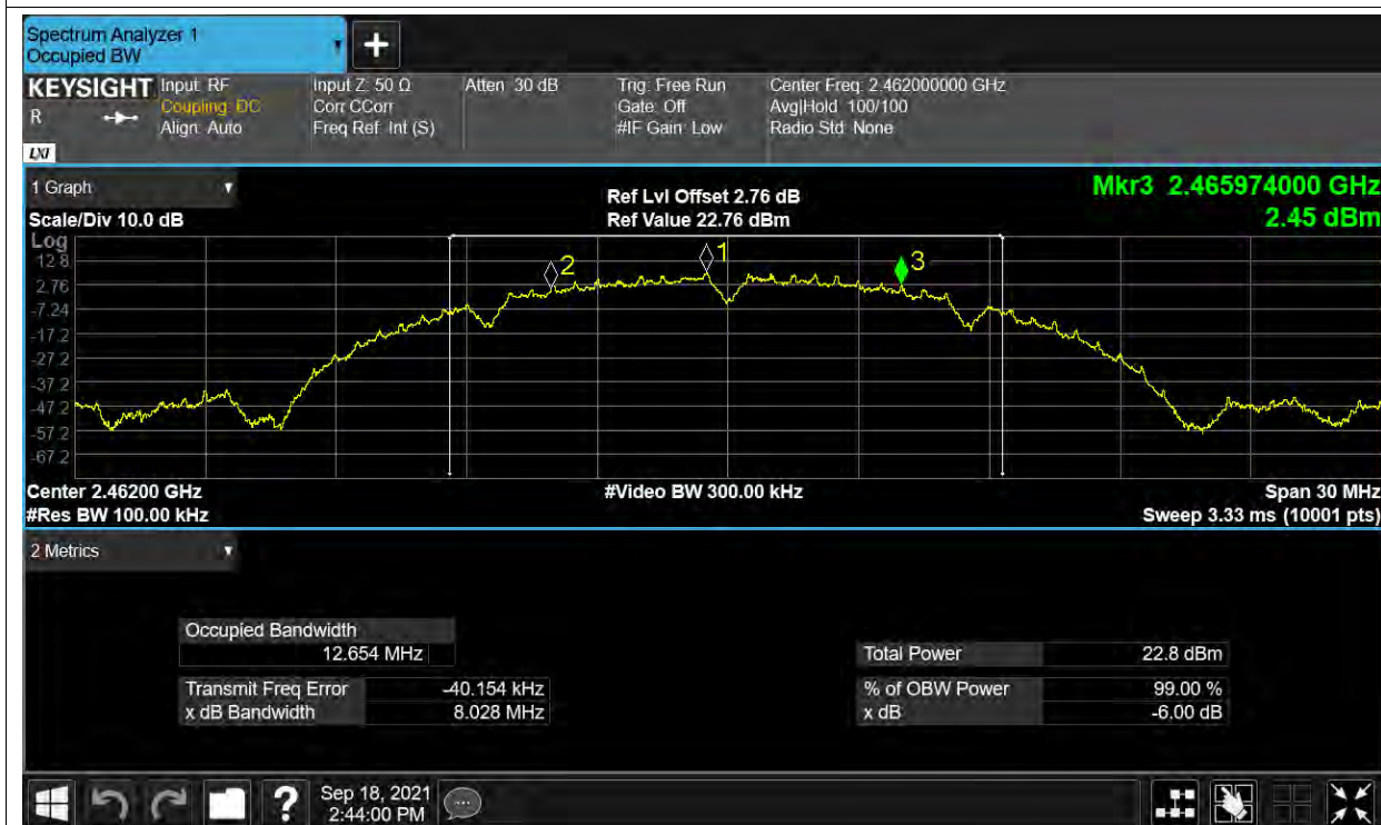
-6dB Bandwidth NVNT g 2412MHz ANT1
