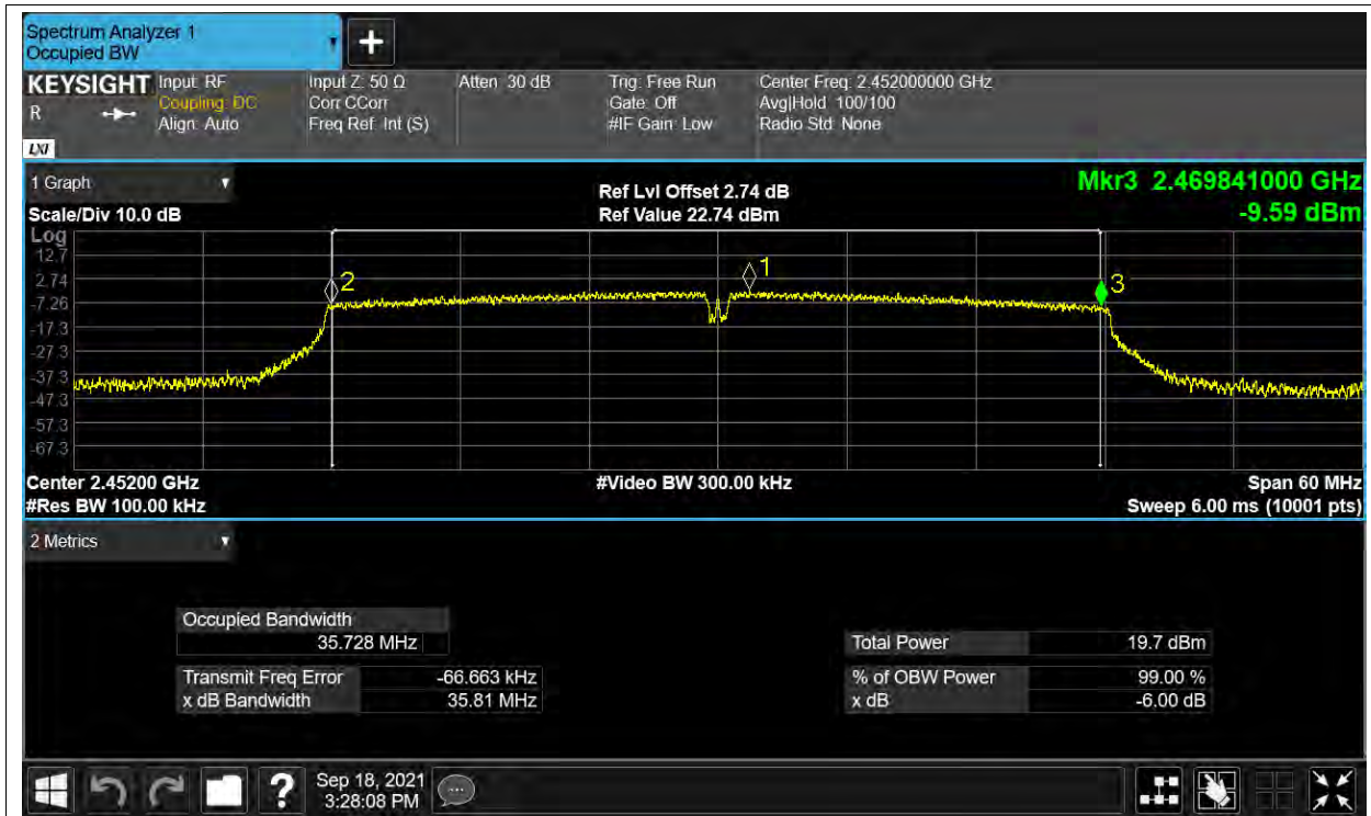
-6dB Bandwidth NVNT n40 2452MHz ANT2
