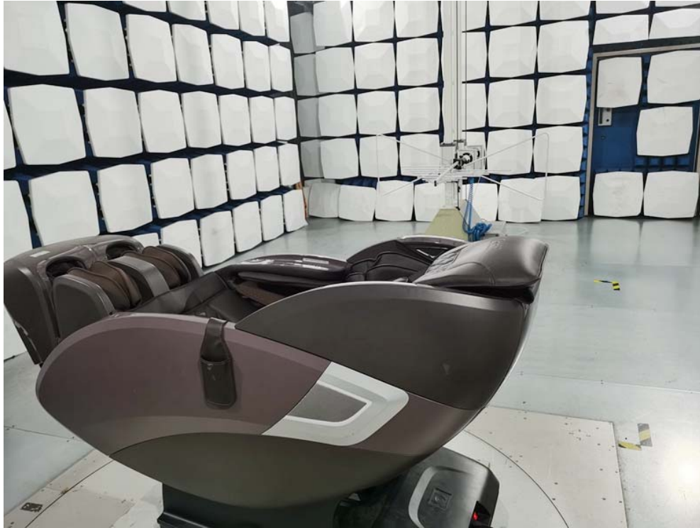
Radiated Emission Test Setup:
