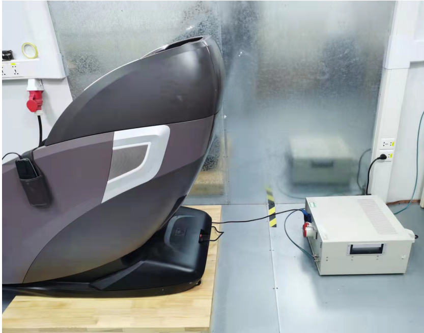
Conducted Emission Test Setup:
