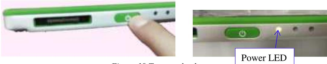
*Figure 19 Turn on the detector*
