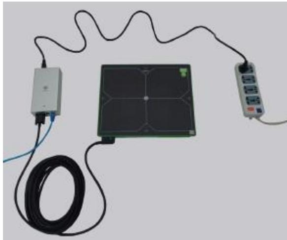
*Figure 37 Wired connection*
