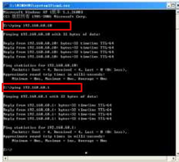
Figure 35 Network testing
