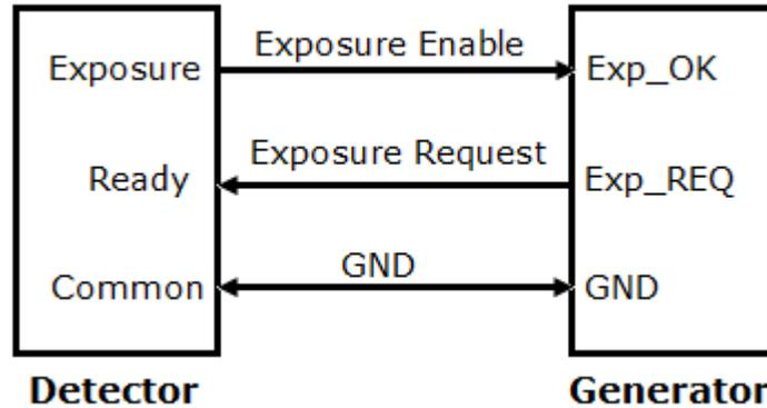
Figure 29 Connection diagram between detector and X-ray generator
