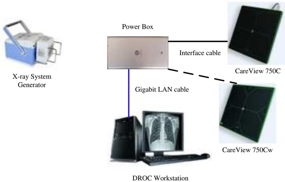
Figure 1 Wired configuration
