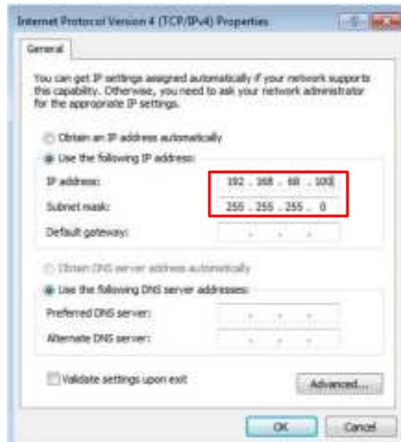
*Figure 33 Set up IP address*
