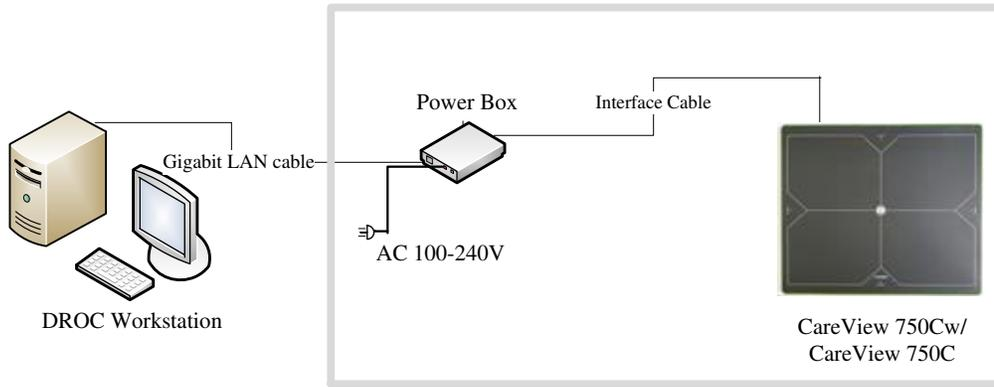
Figure 17 Wired connection (Powered by power box)
