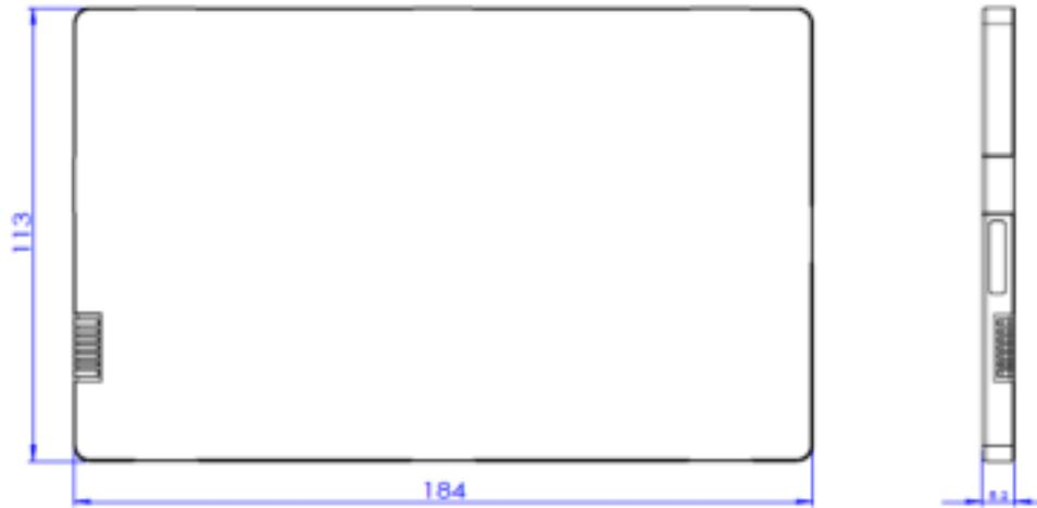
Figure 46 Battery dimension
