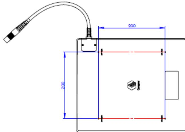
Figure 22 Mounting Holes
