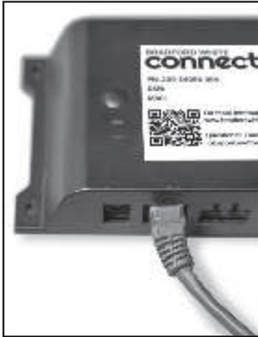
**2.** Plug one end of an ethernet cable into the RJ45 port on the Adapter and another into the RJ45 port on the water heater. Supplied with the Bradford White Connect™ Adapter is a 7 foot CAT5e ethernet cable. Please use either this cable or a similar one, up to a length of 100 feet.
