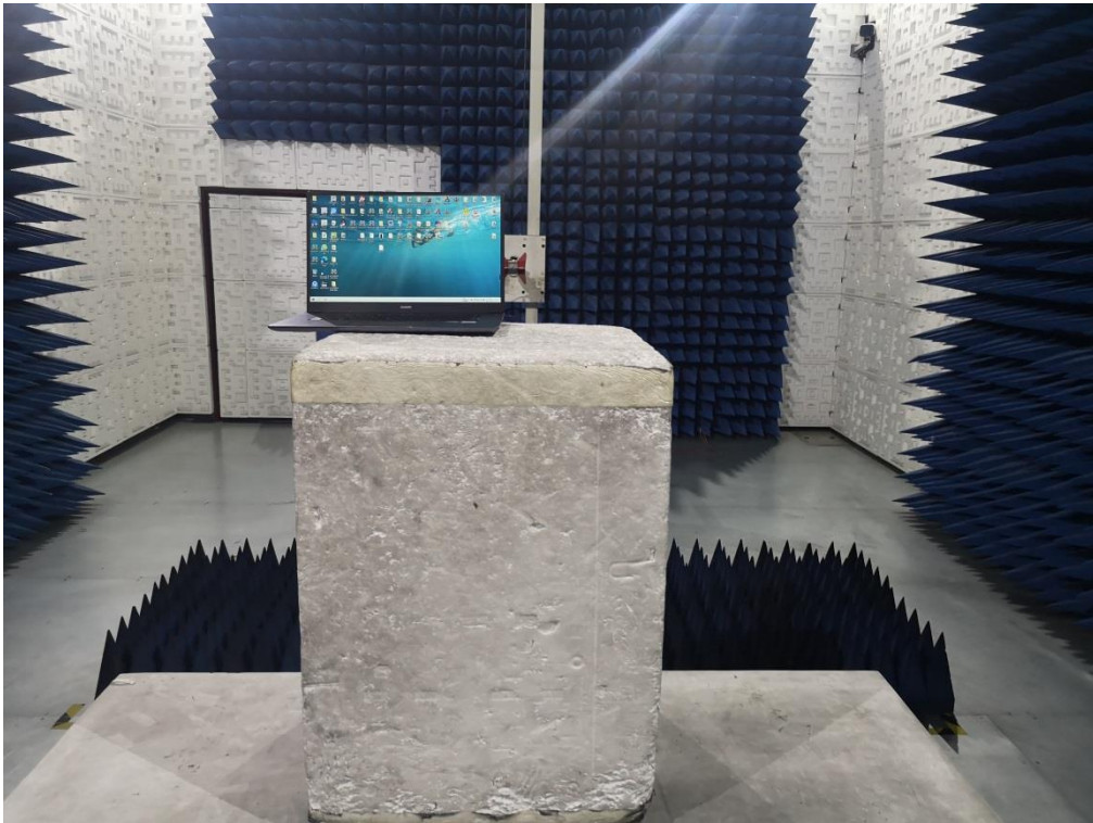
FCC RADIATED EMISSION TEST SETUP ABOVE 1GHZ
