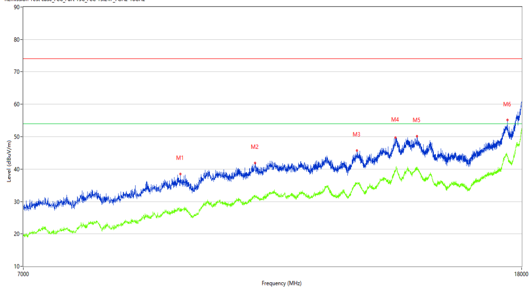
REmission Test case_FCC_Part 15C_FCC 15.247_7GHz-18GHz
