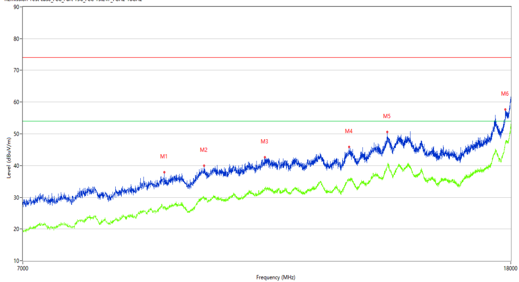
REmission Test case_FCC_Part 15C_FCC 15.247_7GHz-18GHz
