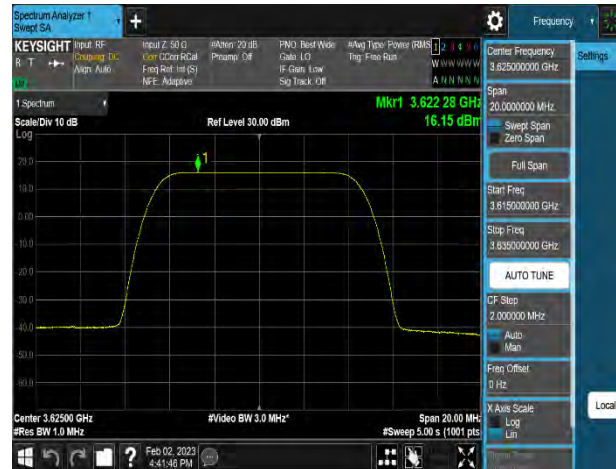
Plot 8-36. Power Spectral Density Plot (n48_1C_10M_16QAM - Mid Channel_8T, Port 2)
