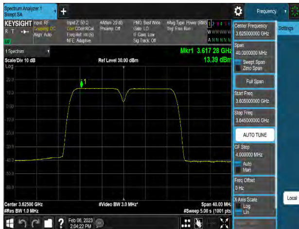
Plot 8-45. Power Spectral Density Plot (n48_2C_10M+10M_QPSK - Mid Channel_8T, Port 3)
