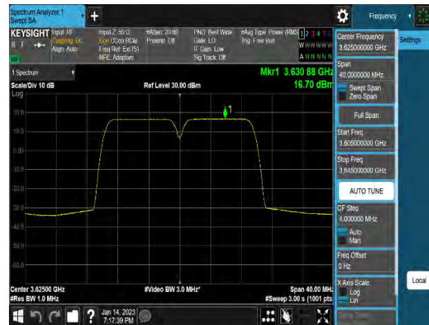
Plot 8-32. Power Spectral Density Plot (n48_2C_10M+10M_16QAM - Mid Channel_4T, Port 6)
