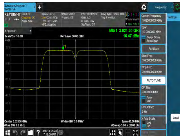
Plot 8-34. Power Spectral Density Plot (n48_2C_10M+10M_16QAM - Mid Channel_4T, Port 8)
