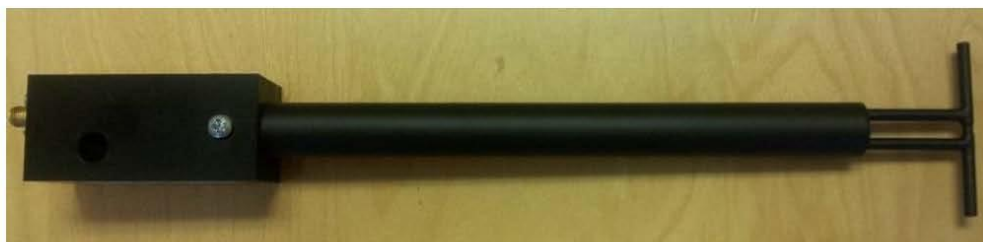
Figure 1 – MVG COMOSAR Validation Dipole
