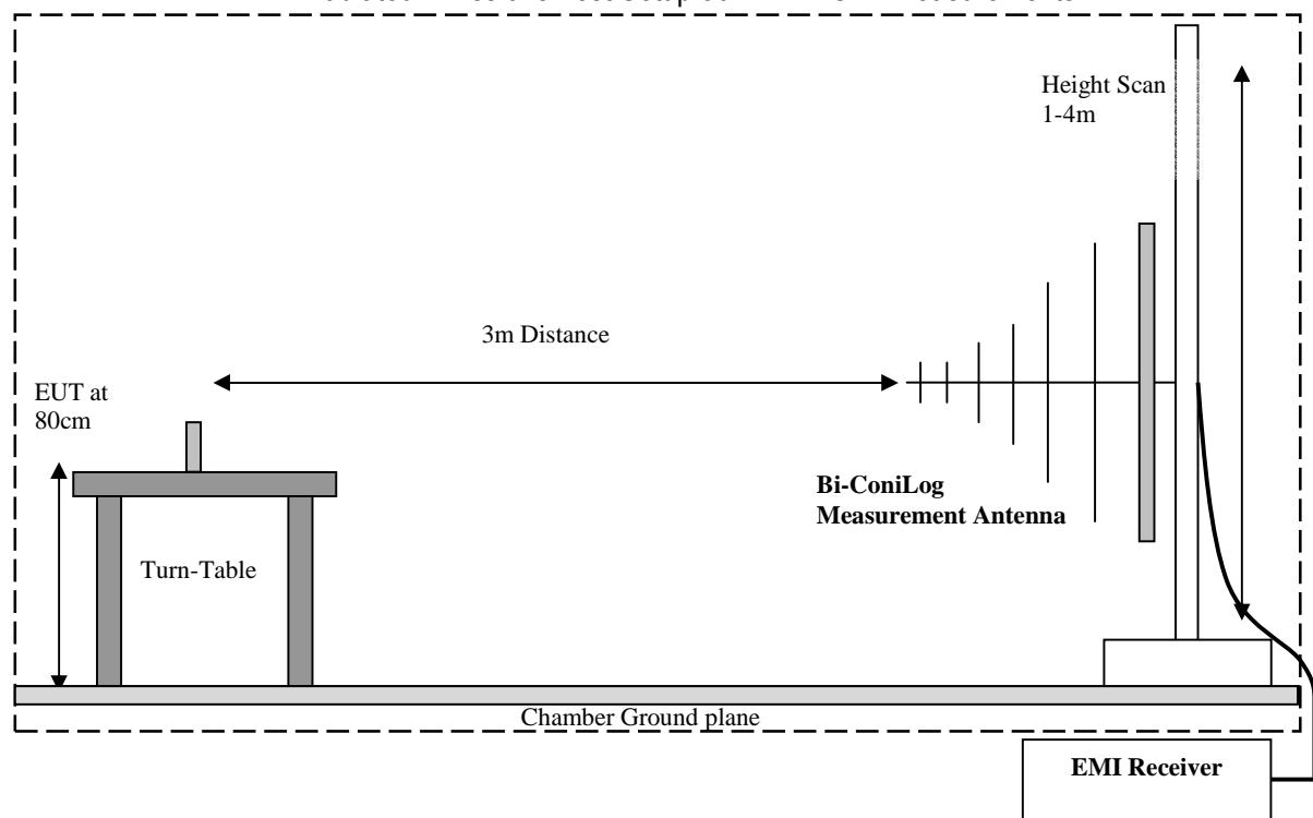
Radiated Emissions Test Setup above 1 GHz Measurements
