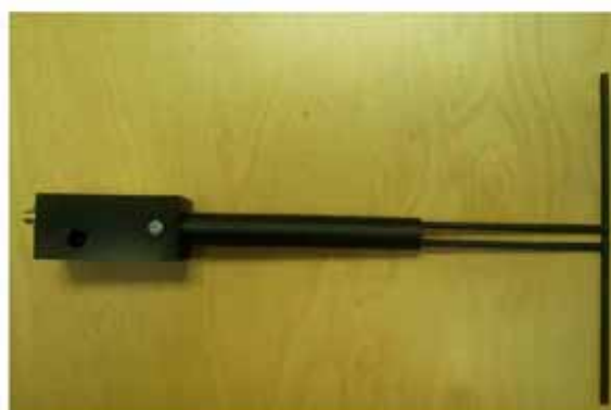
Figure 1 – MVG COMOSAR Validation Dipole
