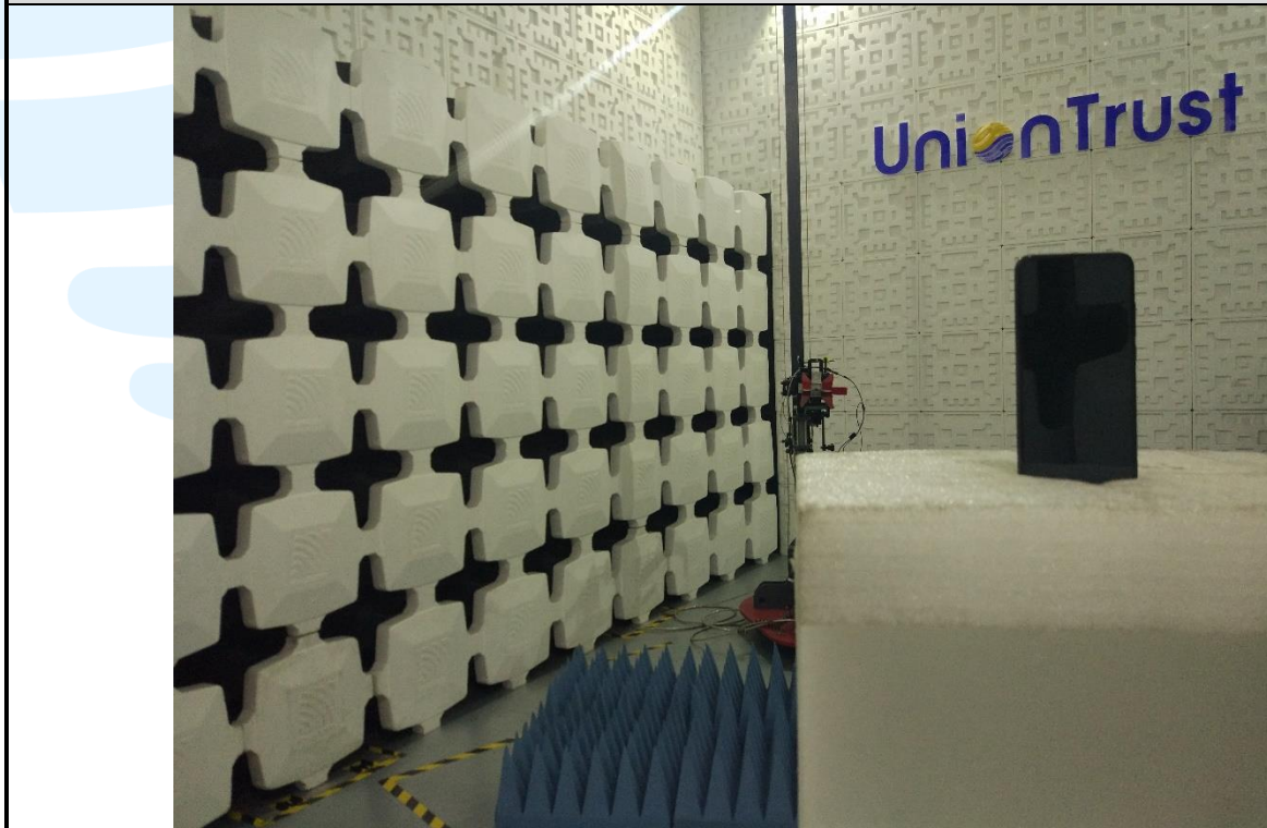
Radiated emission Test Setup (Above 1 GHz)
