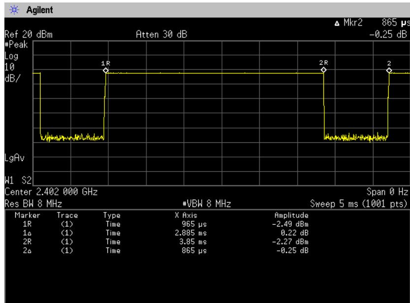
$$\text{Duty Cycle} = \text{Ton} / (\text{Ton} + \text{Toff}) = 2885[\mu\text{s}] / (2885[\mu\text{s}] + 865[\mu\text{s}]) = 76.93\%$$
