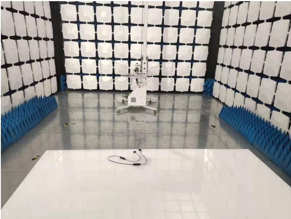
Below 1GHz for radiated emission test setup
