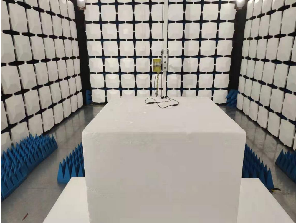
Above 1GHz for radiated emission test setup
