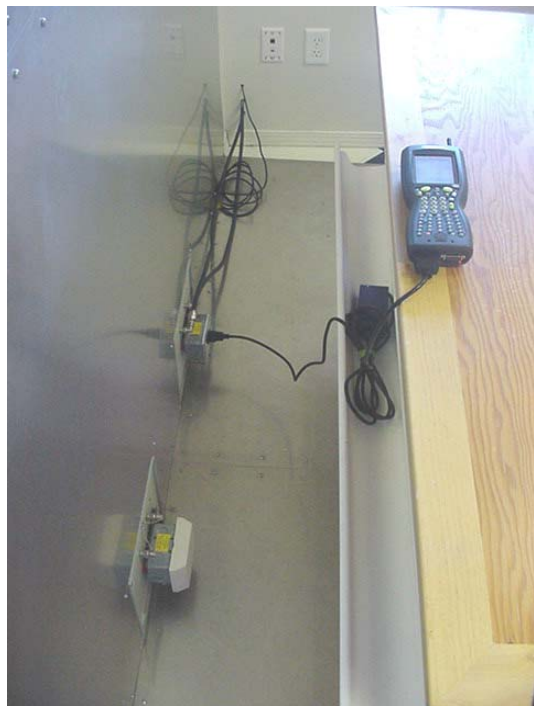
Photograph F-1 - AC Powerline Conducted Emission Cable Placement
