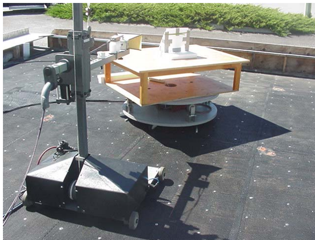
Photograph C-2 - Horn Receive Antenna in Vertical Polarization
