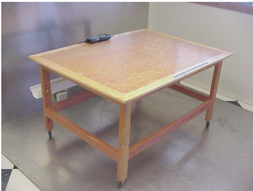
Photograph F-2 - AC Powerline Conducted Emission Configuration
