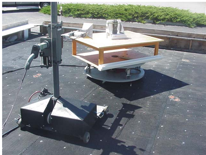
Photograph C-1 - Horn Receive Antenna in Horizontal Polarization
