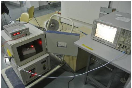
Radiated Spurious Measurement(below 30MHz) Setup
