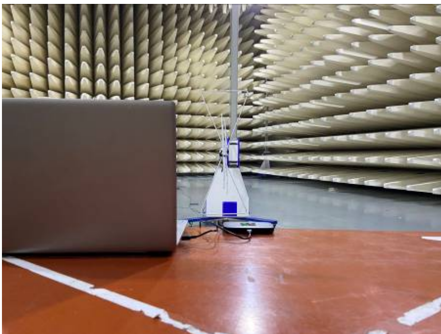
Radiated Emissions Test Setup (with laptop) (30-1000MHz)
