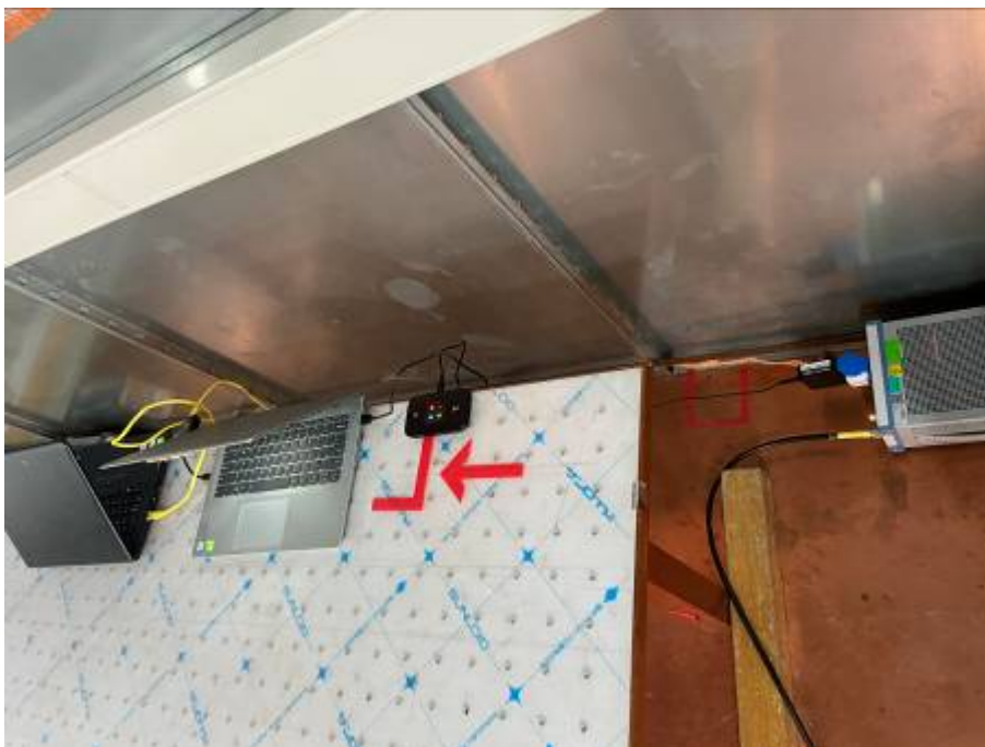
Conducted Emissions Test Setup (with laptop)
