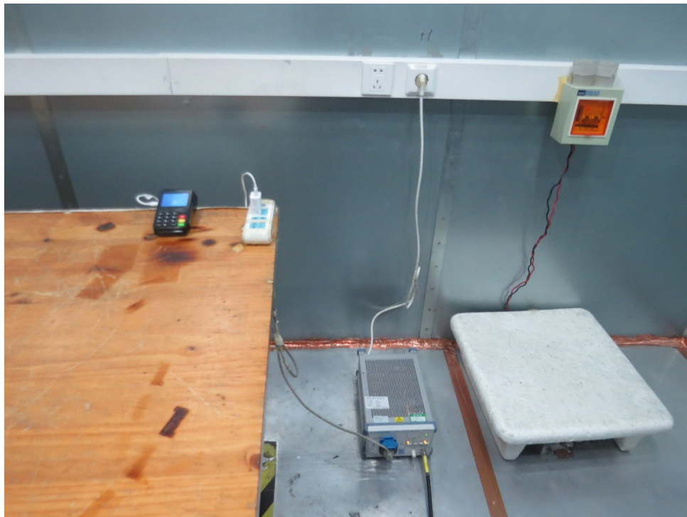
Picture 2 Conducted Emission Test Setup
