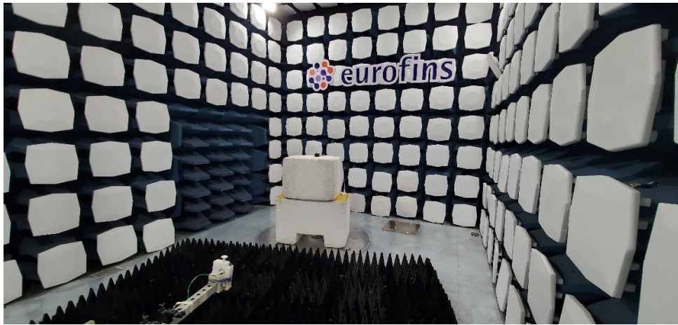
Picture 1 Radiated Emission Test Setup
