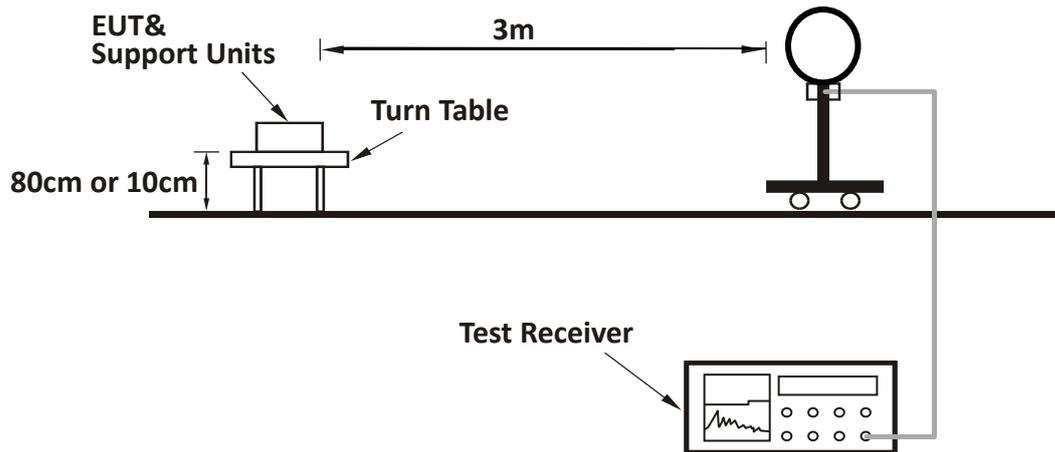
For Radiated emission 30MHz to 1GHz:
