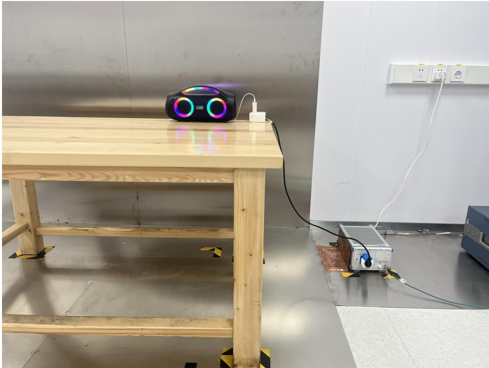
Radiated Emission Test View|(Below 1G)
