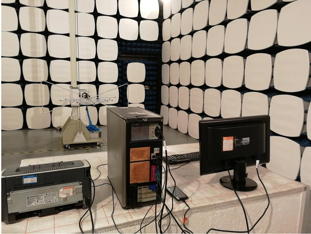
Radiated Emission Below 1GHz
