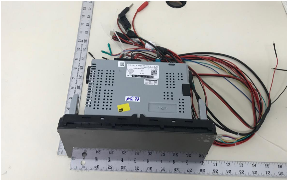
Figure F1: Conducted DUT Set up
