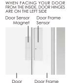
When you are installing the Door Sensor, make sure the arrows on the Door Sensor is placed next to the arrow from the Door Frame
