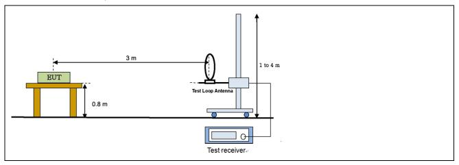
Radiated emission setup, Below 1 000 MHz
