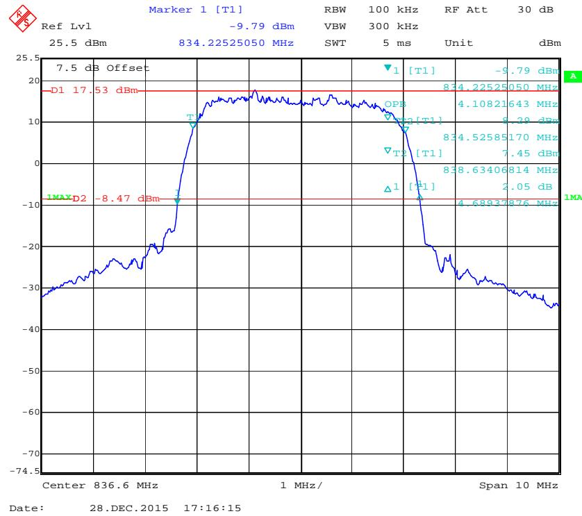
**PCS Band (Part 24E)****99% & 26 dB Occupied Bandwidth for GSM (GMSK) Mode**
