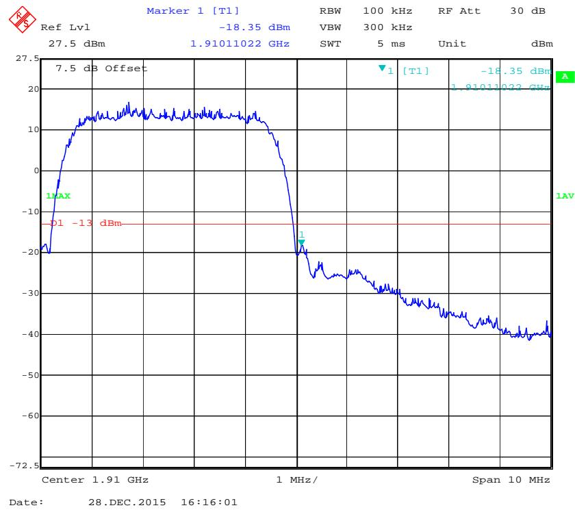
**PCS Band, Left Band Edge for HSUPA (BPSK) Mode**
