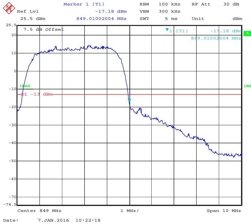
**Cellular Band, Left Band Edge for HSDPA (16QAM) Mode**
