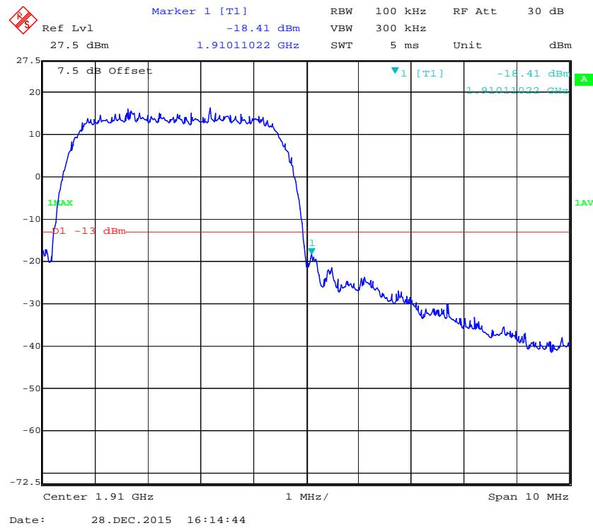
**PCS Band, Left Band Edge for HSDPA (16QAM) Mode**
