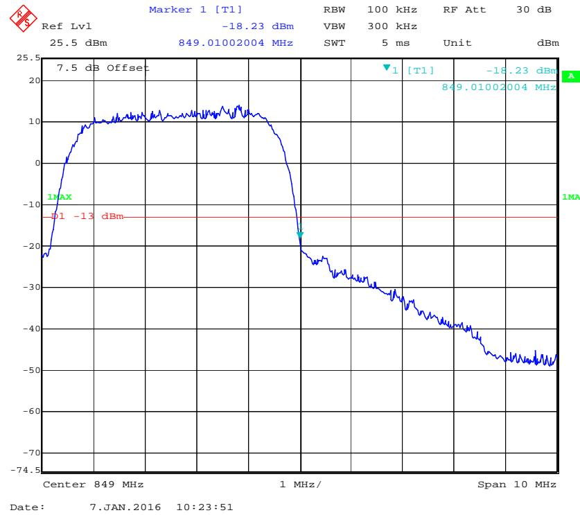
**PCS Band, Left Band Edge for GSM (GMSK) Mode**
