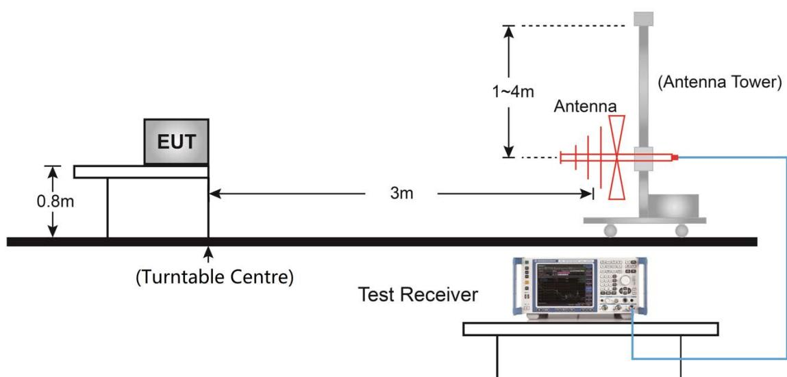
Above 1GHz Test Setup:
