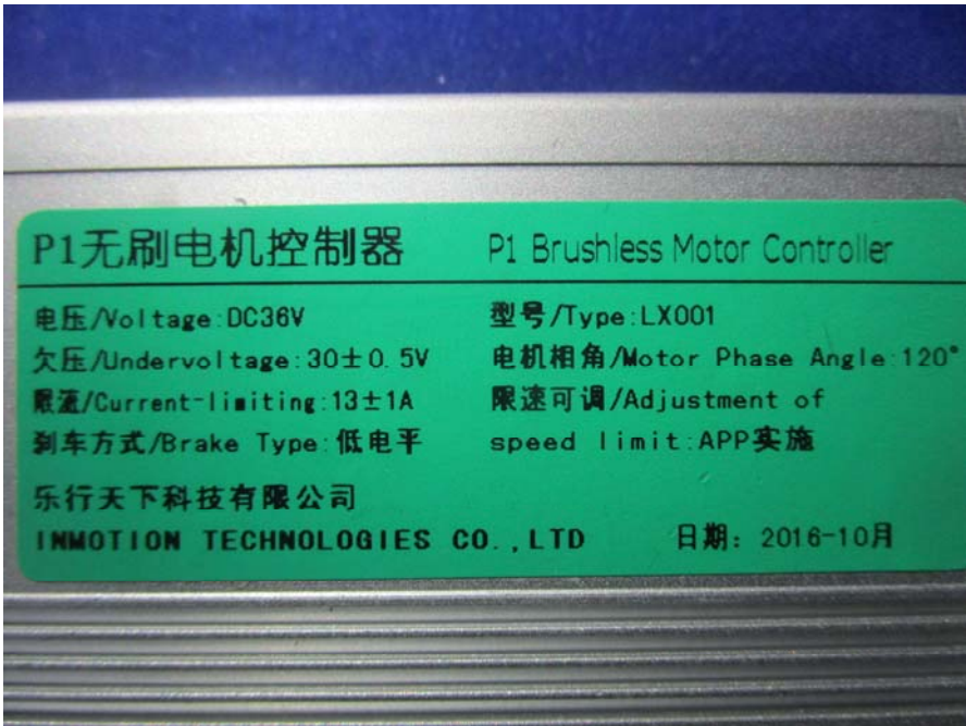
EUT – Motor Controller Label View
