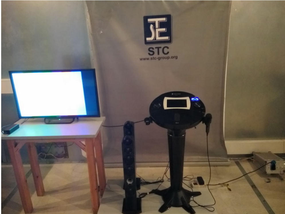
Measurement of Conducted Emission Test Set Up
