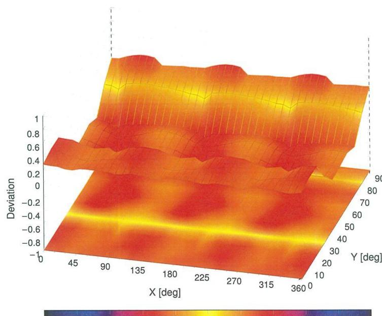
Probe isotropy for  $E_{\text{tot}}$ : probe rotated  $\phi = 0^\circ$  to  $360^\circ$ , tilted from field propagation direction  $\vec{k}$
