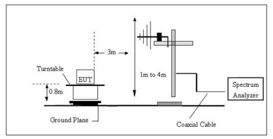
(C) Radiated Emission Test-Up Frequency Above 1GHz
