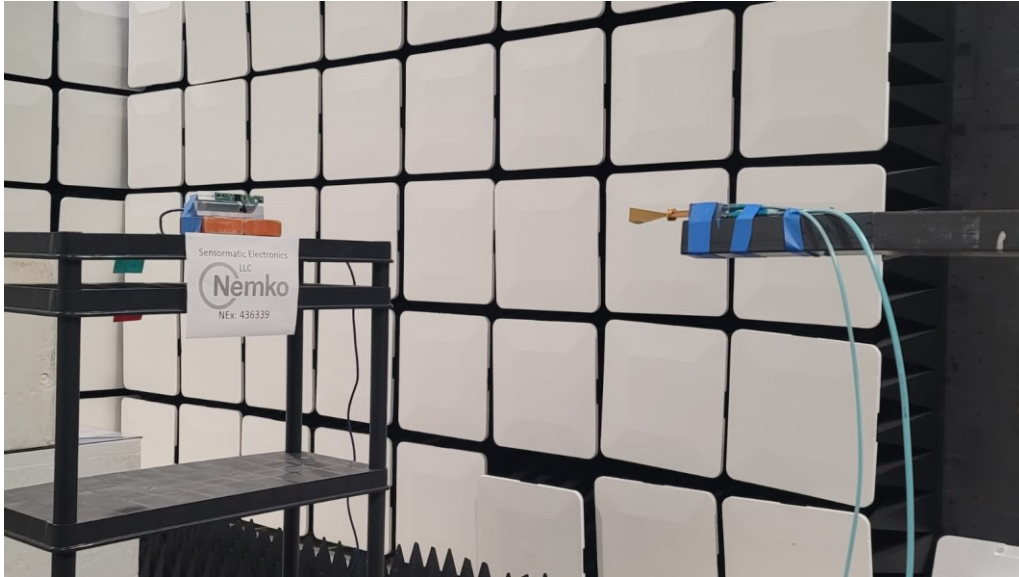
Figure 11 - Radiated emissions above 1 GHz (75 – 110 GHz), front view, 1 meter distance.
