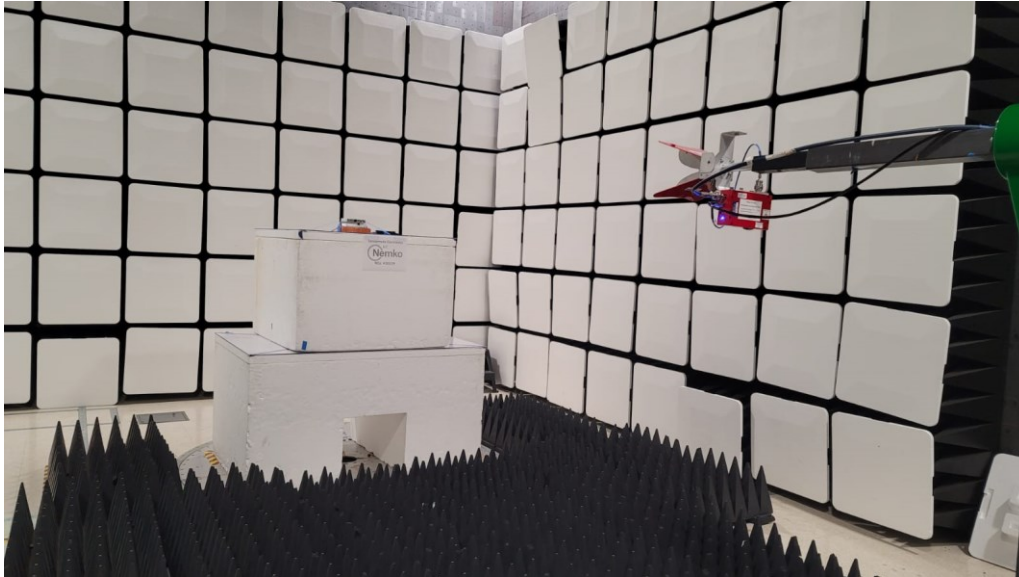
Figure 3 - Radiated emissions above 1 GHz (1 – 18 GHz), front view, 3 meters distance.
