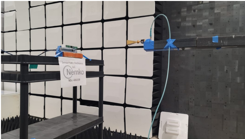
Figure 14 – Test setup (power meter measurements, 0.47 meters distance).
