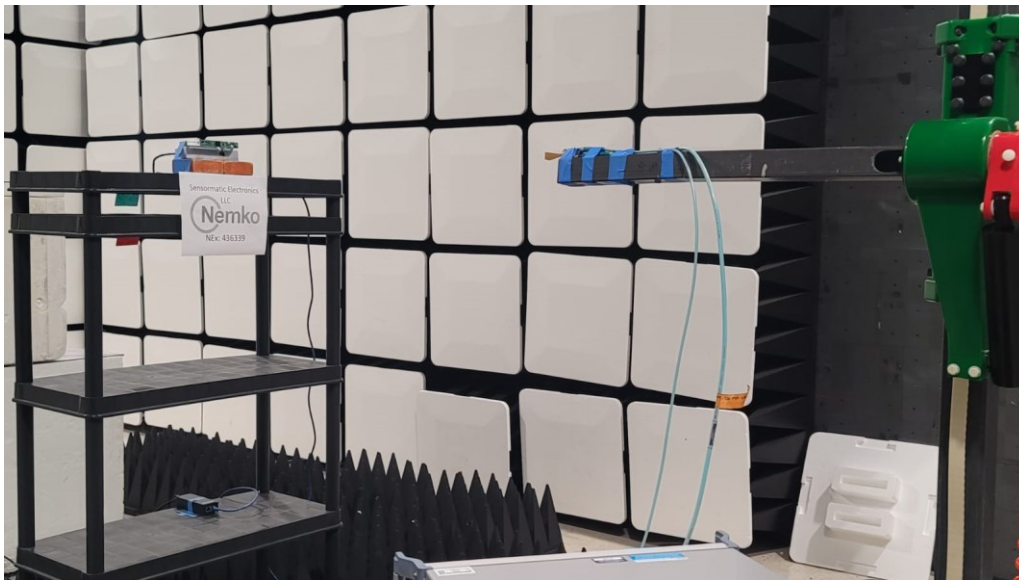
Figure 12 - Radiated emissions above 1 GHz (110 – 140 GHz), front view, 1 meter distance.
