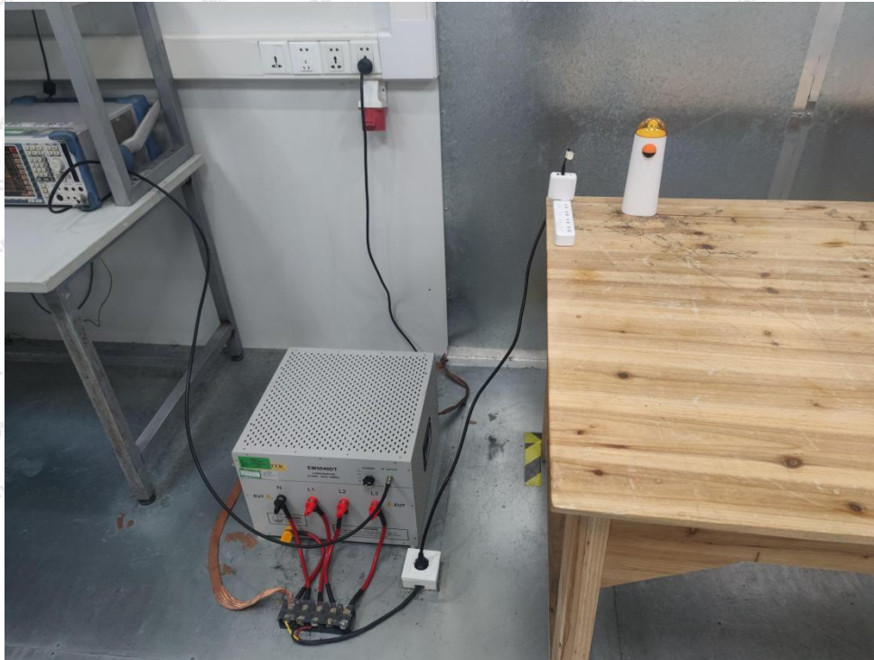
Photo of Conducted Emission Measurement
