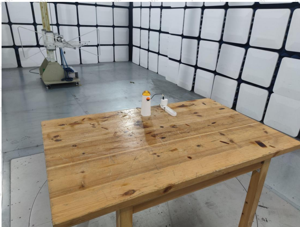
Photo of Radiation Emission Test
