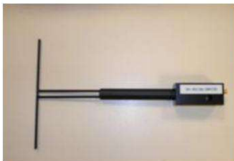
Figure 1 – Satimo COMOSAR Validation Dipole
