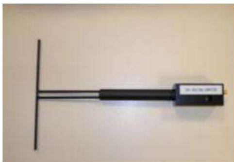
Figure 1 – Satimo COMOSAR Validation Dipole
