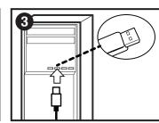
**3.** Plug the USB charging cable into a 5V DC computer outlet.
