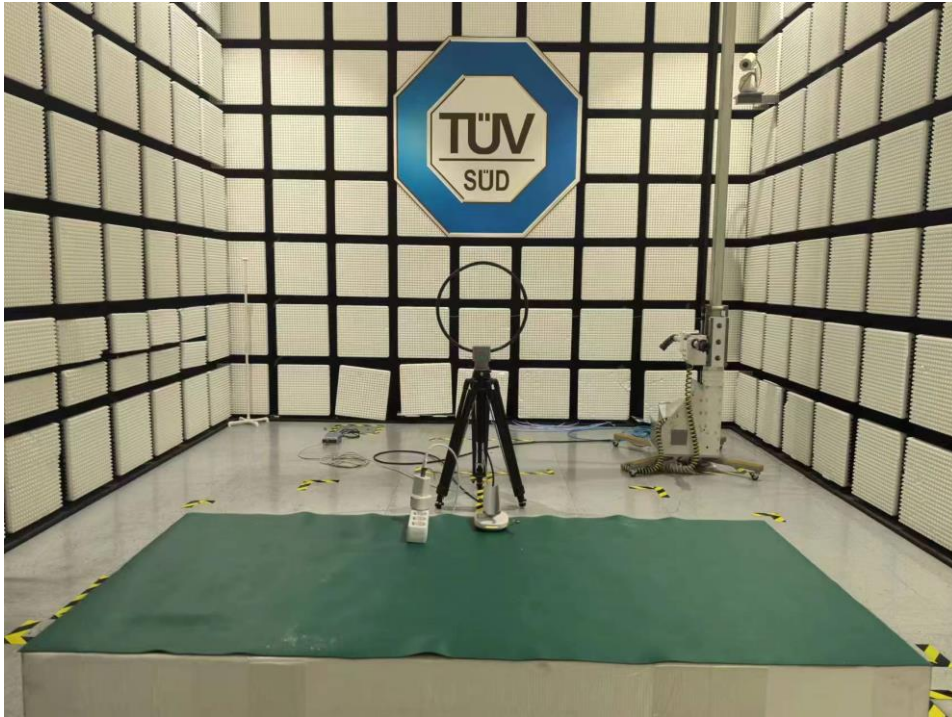
Radiated Emission Setup 9kHz ~ 30MHz
