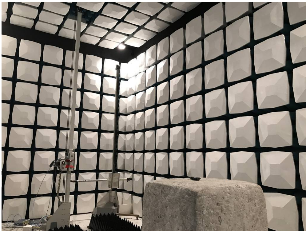
Description: Radiated Emission Test Setup for 1~18GHz
