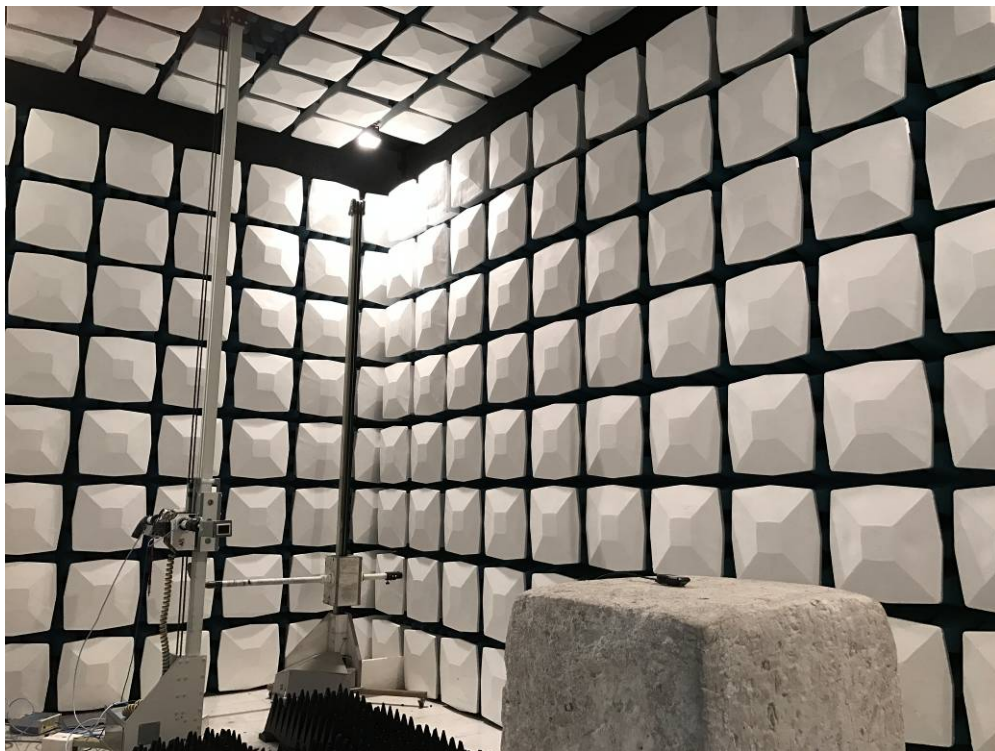
Description: Radiated Emission Test Setup for 18-40GHz
