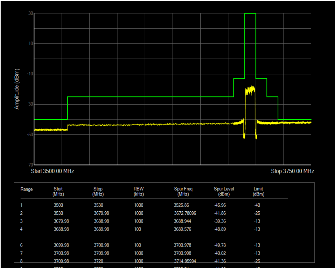
n78(3550-3700) SCS=30kHz CP_QPSK BW=10MHz Channel=646332 RB=1@23
