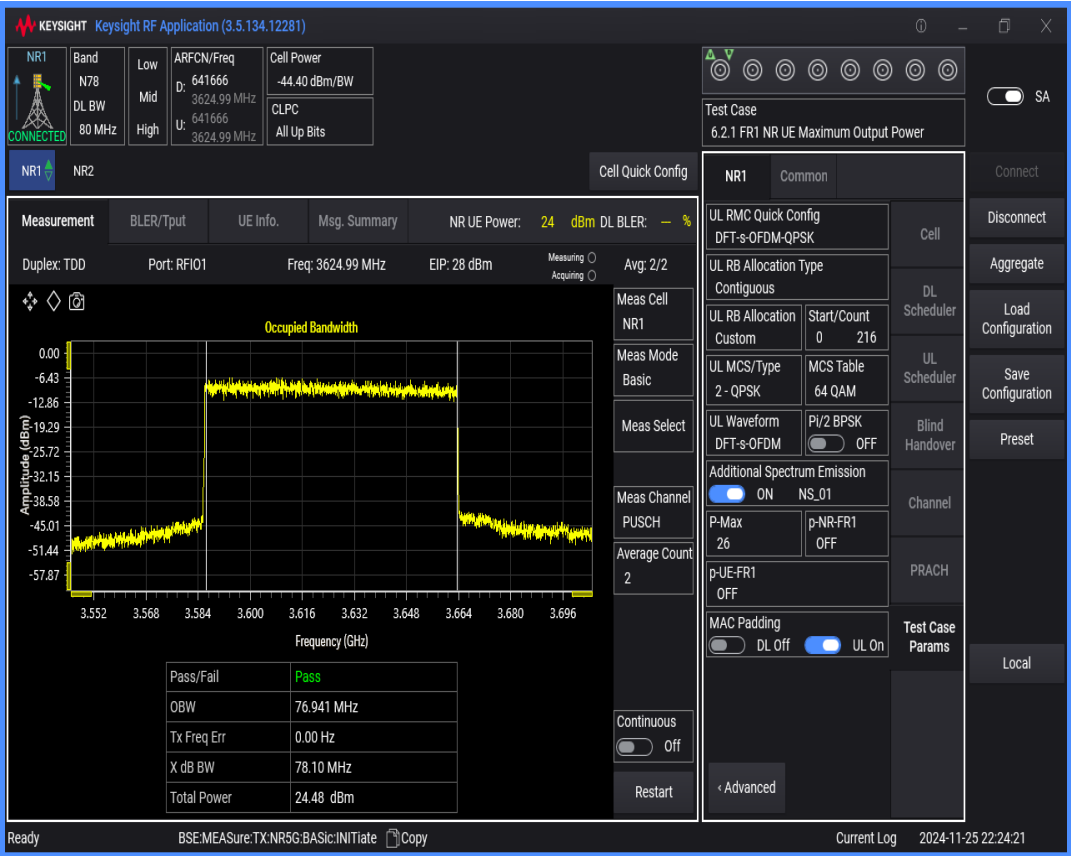
n78(3550-3700) SCS=30kHz DFT_QPSK BW=70MHz Channel=641666 RB=180@0
