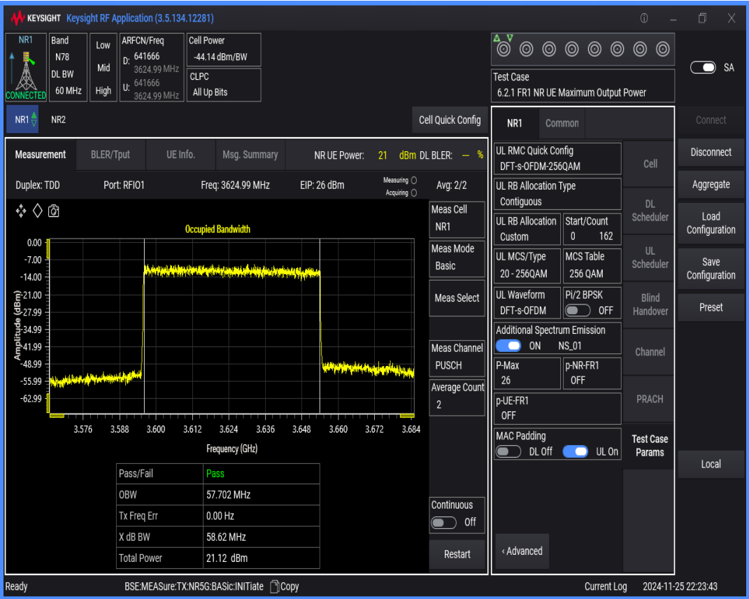
n78(3550-3700) SCS=30kHz DFT_QAM256 BW=70MHz Channel=641666 RB=180@0
