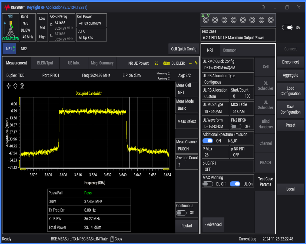
n78(3550-3700) SCS=30kHz DFT_QAM64 BW=50MHz Channel=641666 RB=128@0
