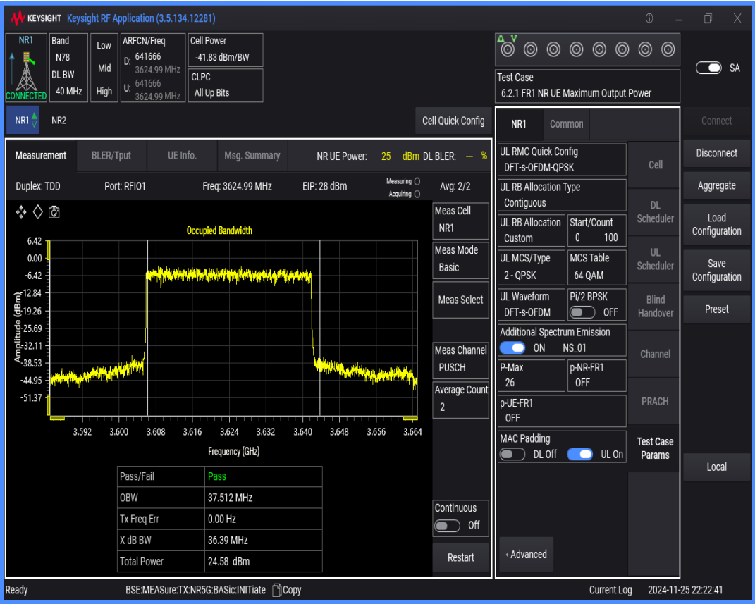
n78(3550-3700) SCS=30kHz DFT_QPSK BW=60MHz Channel=641666 RB=162@0
