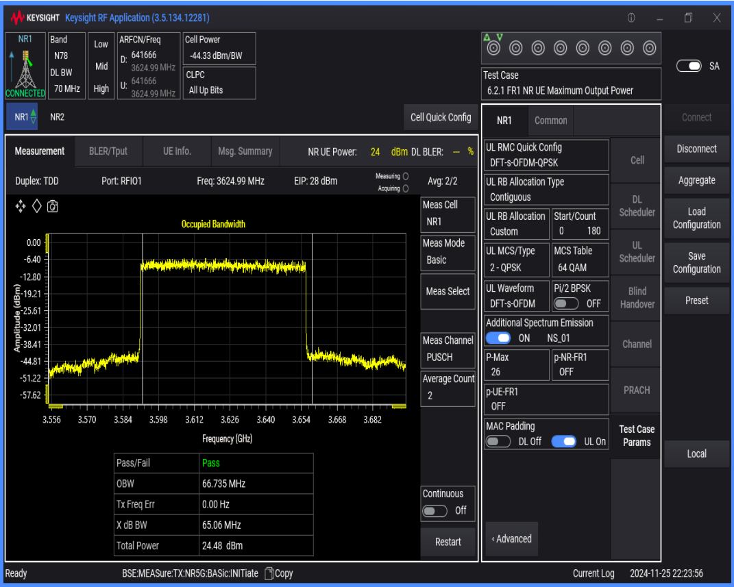
n78(3550-3700) SCS=30kHz DFT_QPSK BW=90MHz Channel=641666 RB=240@0
