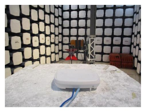
1.4 Radiated Spurious Emission 1-18 GHz Rear View, 1 meter
